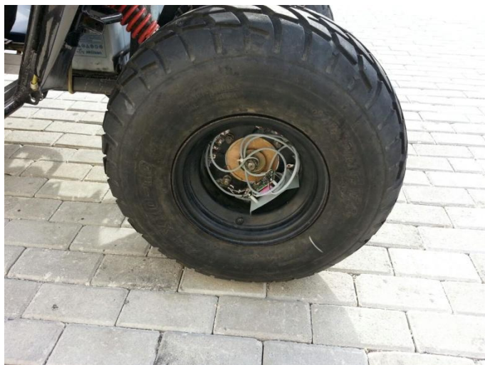
Figure 5.20 Telemetry circuit and the rim is attached on the vehicle
