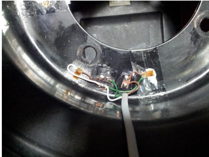
Figure 5.18 Quarter bridge type-II installation of strain gauges
