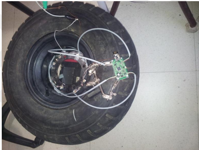
Figure 5.19 Installation of the transmitter circuit on the rim
