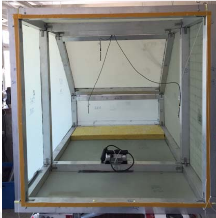
Figure 5.20 Manufactured cabinet model a) cabinet, b) position of vibration motor and damping material (continued)
