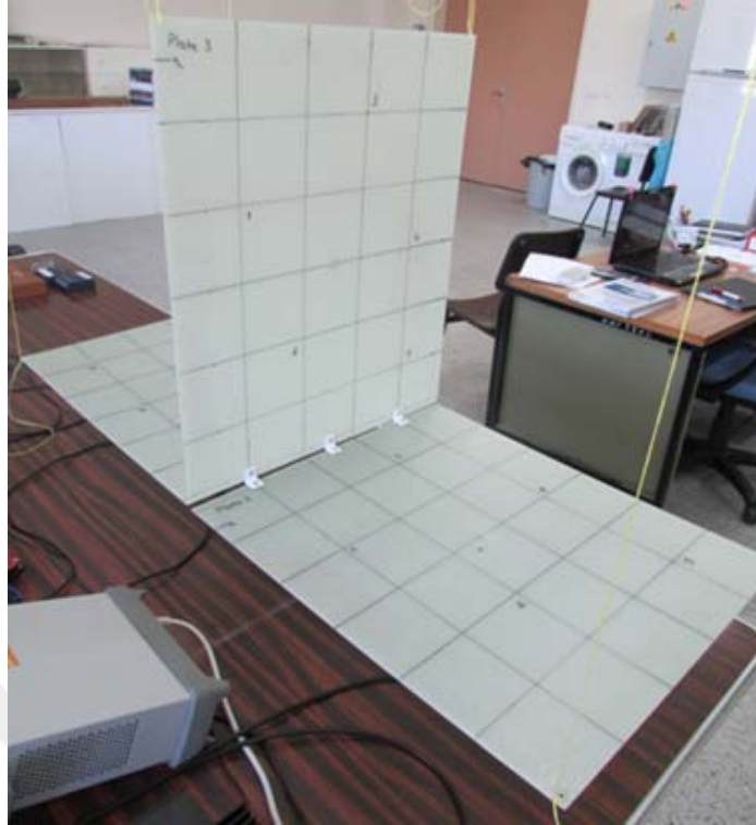
Figure 3.6 T-type structure with point connections
