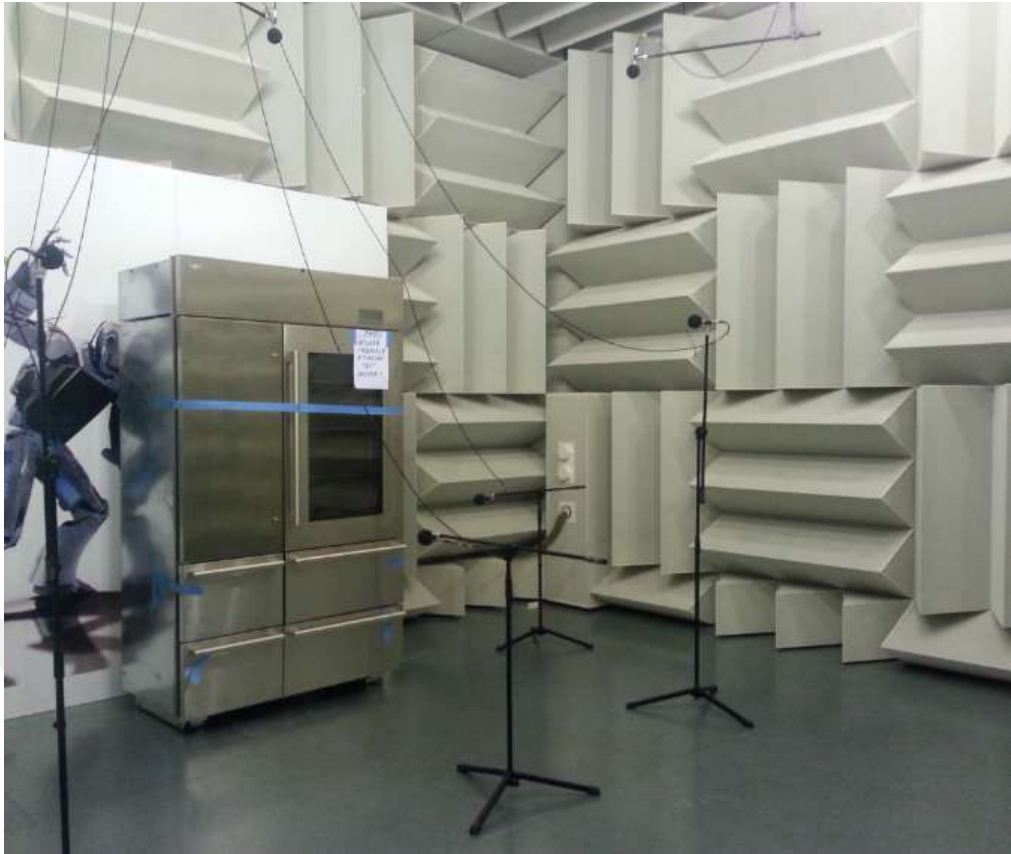
Figure 3.1 Sound measurement of a refrigerator in semi-anechoic room
