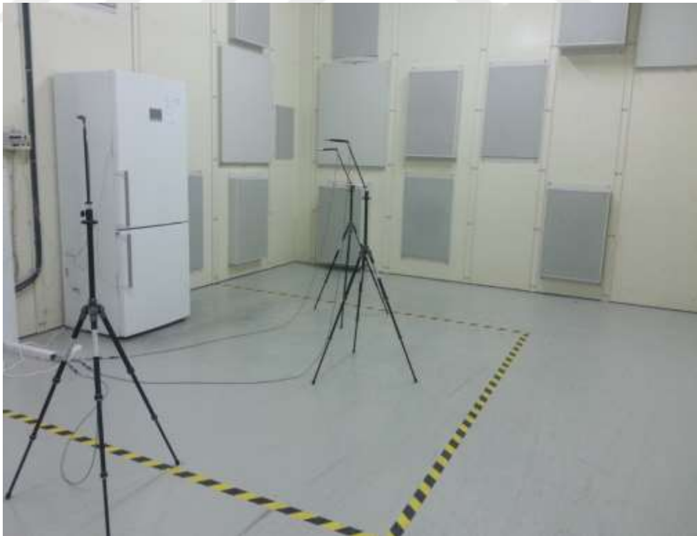
Figure 3.2 Sound measurement of a refrigerator in reverberation room
