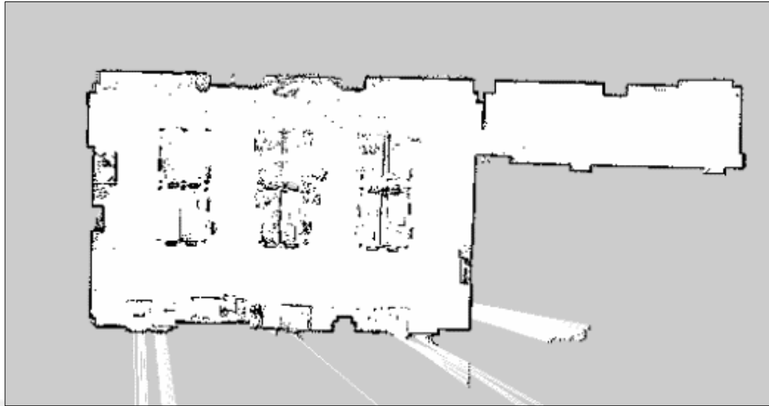
Figure 4.20 Built map of DEU Automatic Control Laboratory and its corridor
