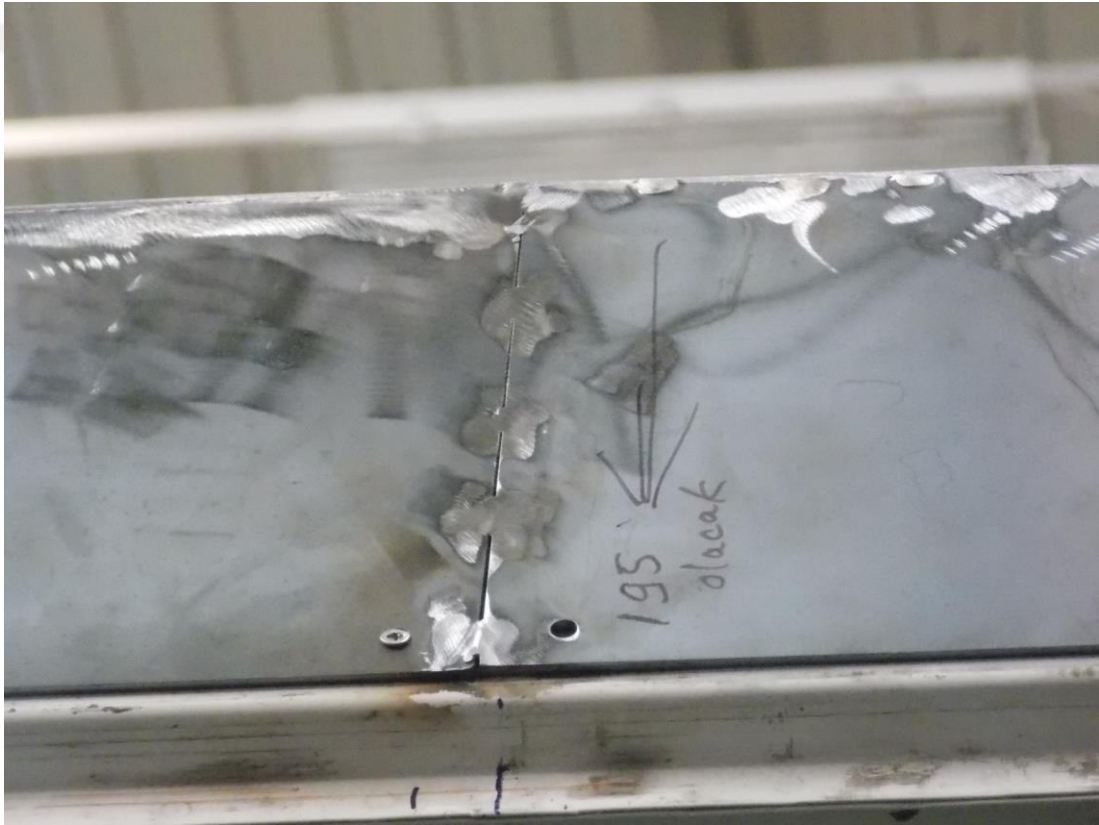
Figure 3.1 MAG welding on Ramor500 armor steel.
