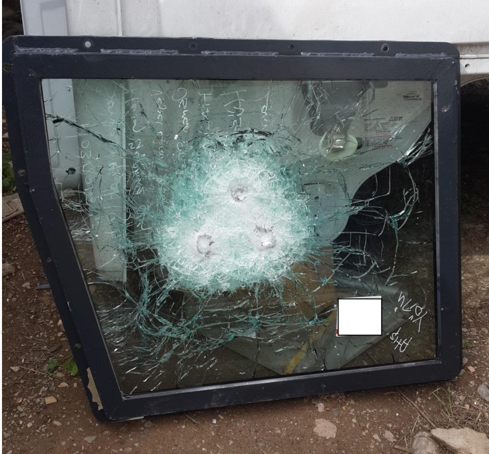
Figure 4.1 Test result of armor glass according to BR6.
