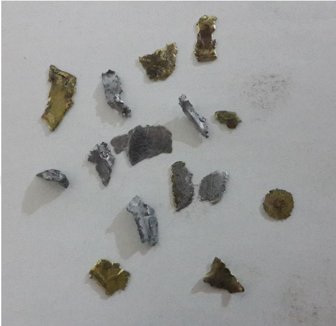
Figure 5.10 Deformed bullet after ballistic test.
