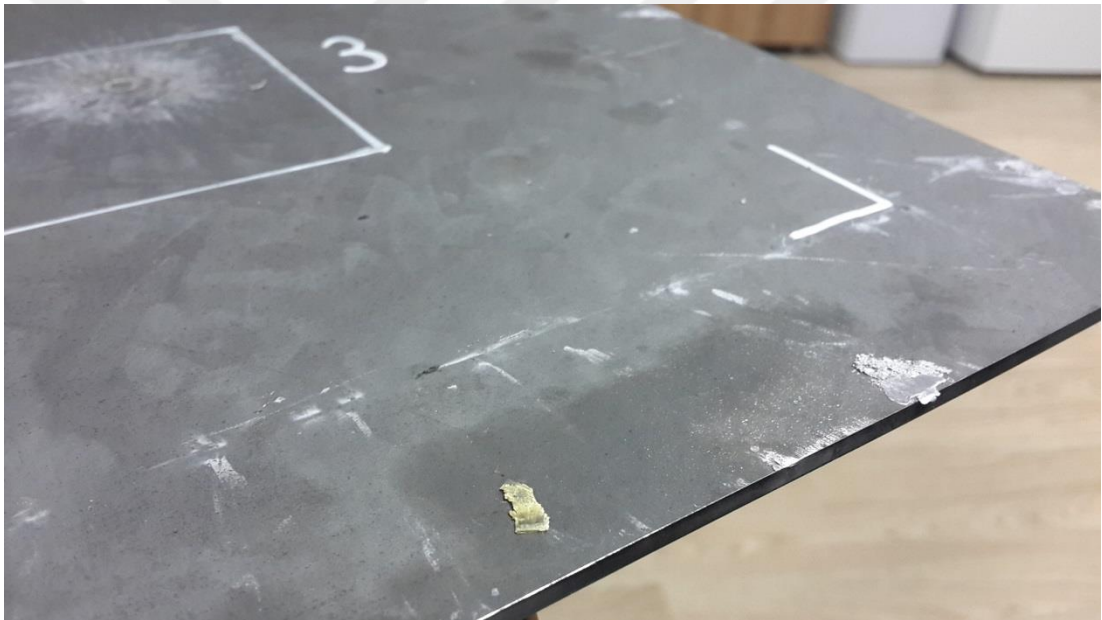
Figure 5.9 Sticked particles between the target and holding jaws.
