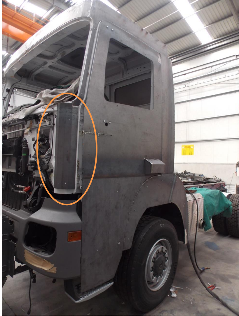
Figure 3.2 Ramor500 plate bended 30° for three times.
