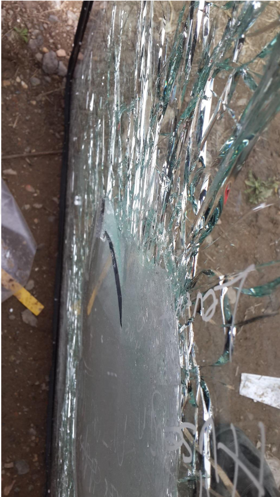
Figure 4.1 Test result of armor glass according to BR6 (continue).
