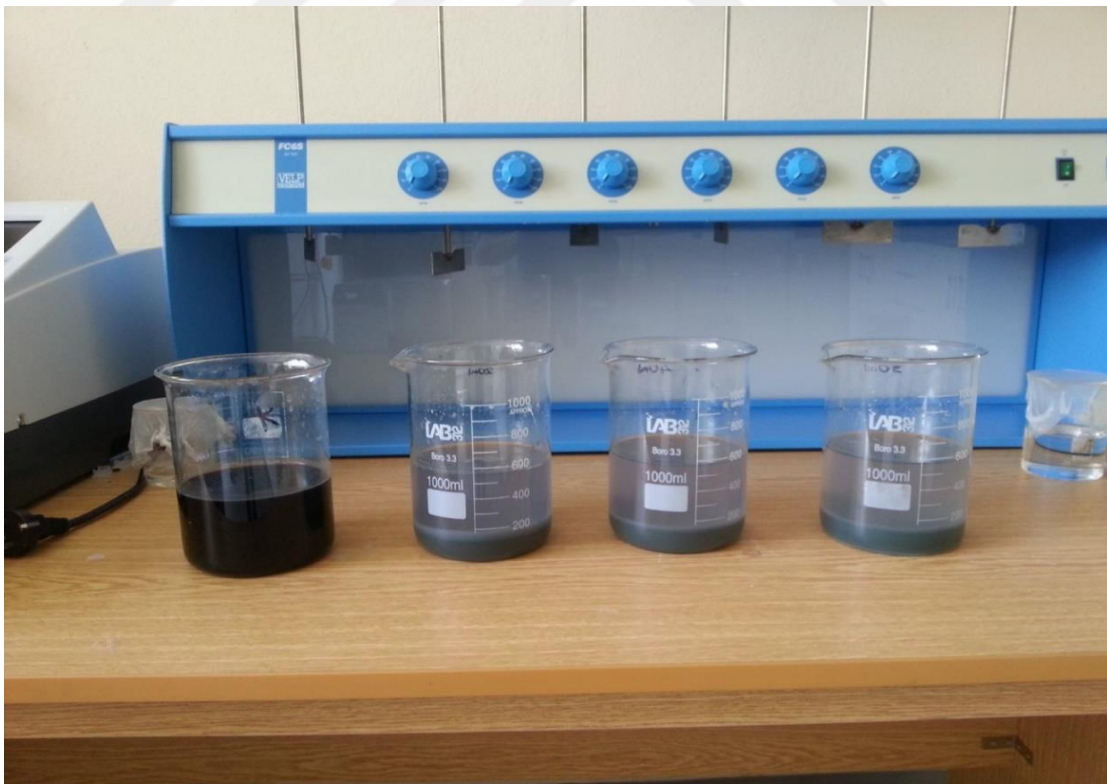
Figure 5.7 Jar testing kits and \text{MgO} application image
