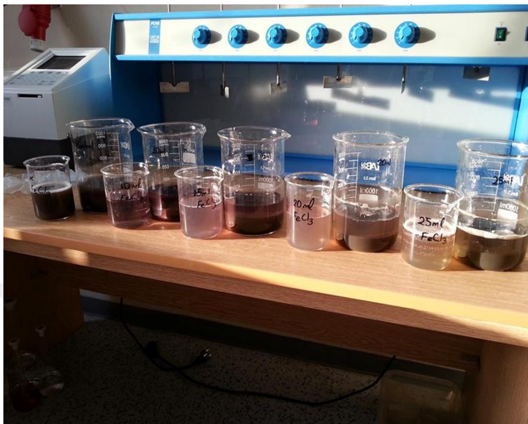
Figure 5.2 Jar testing kits and FeCl 3 application image
