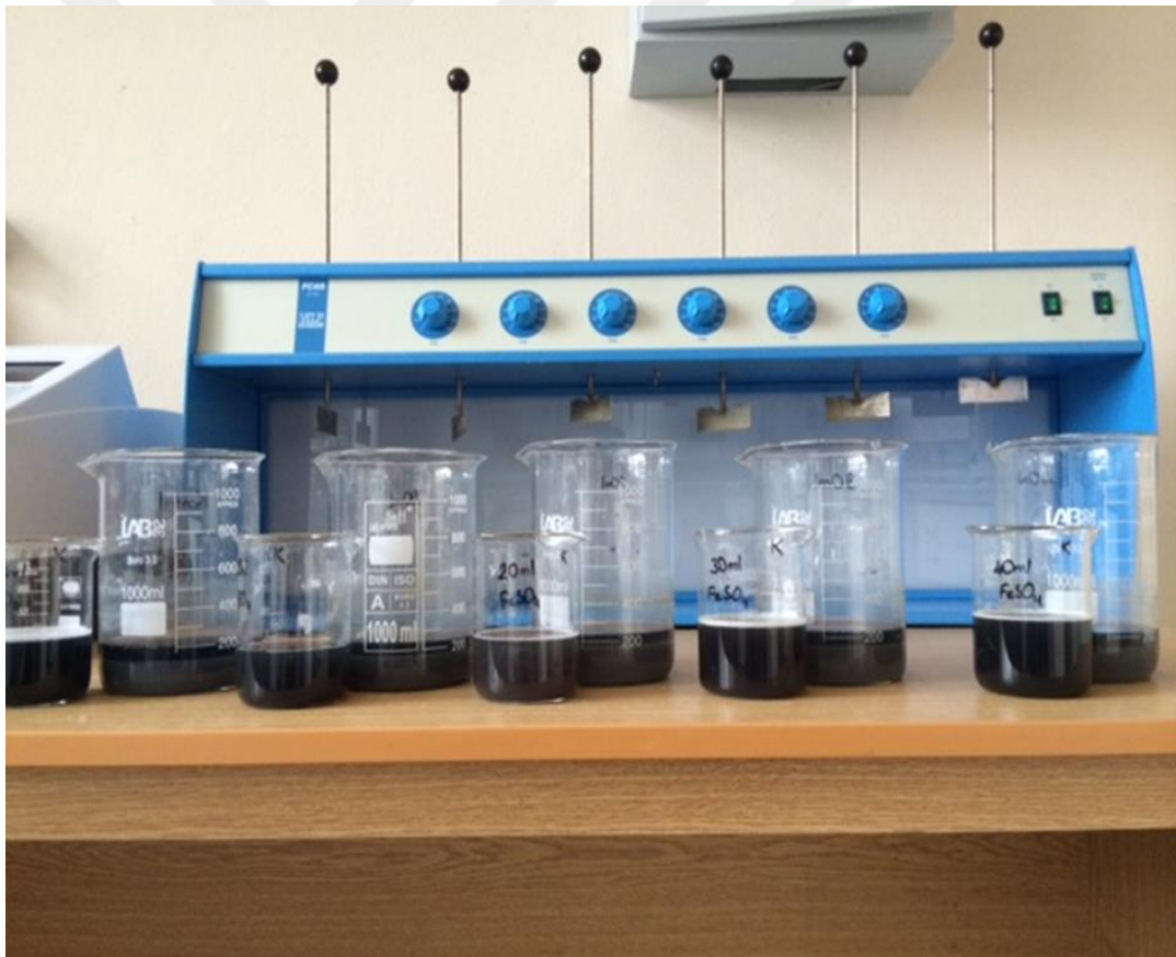
Figure 5.4 Jar testing kits and FeSO 4 application image
