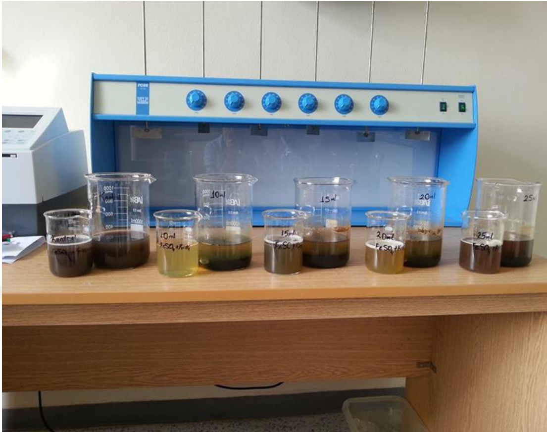
Figure 5.1 Jar testing kits and FeSO 4 application image
