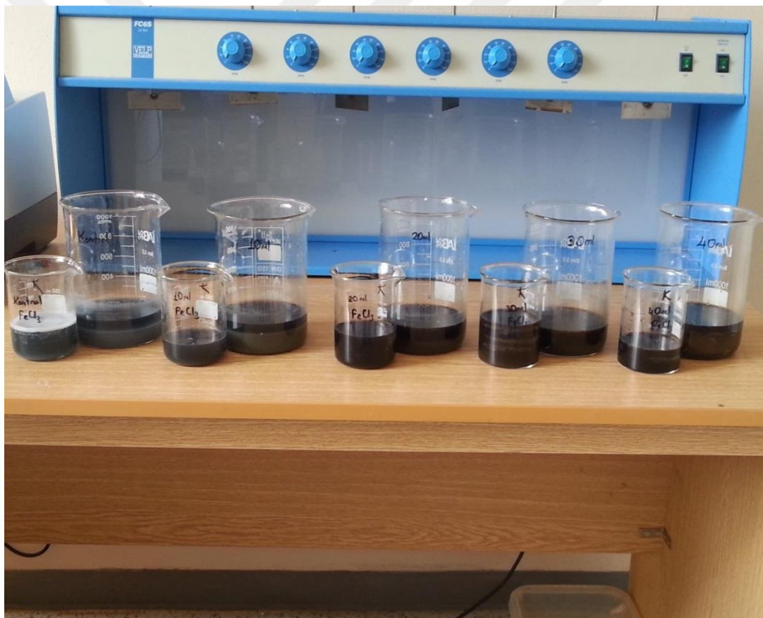
Figure 5.5 Jar testing kits and FeCl 3 application image
