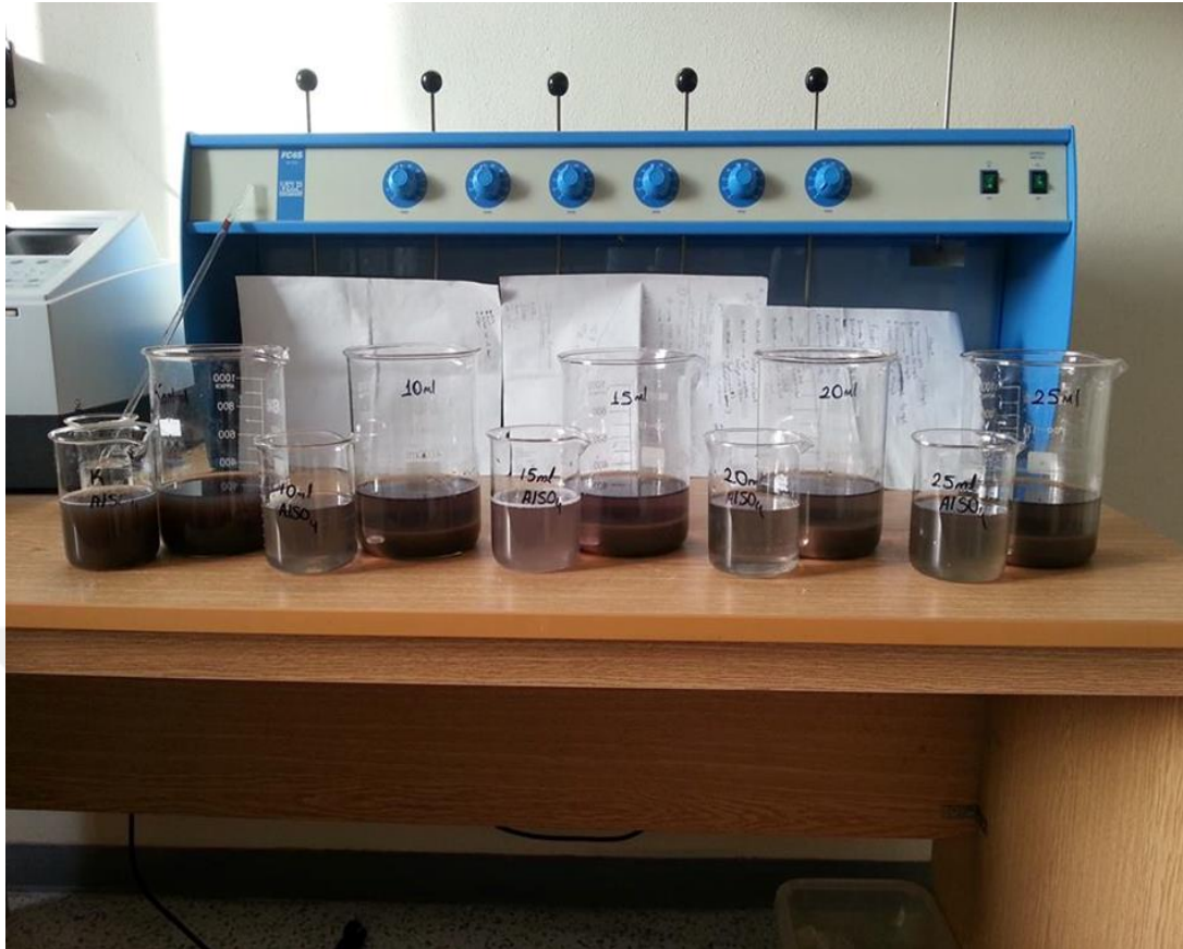
Figure 5.3 Jar testing kits and \text{Al}_2(\text{SO}_4)_3 application image
