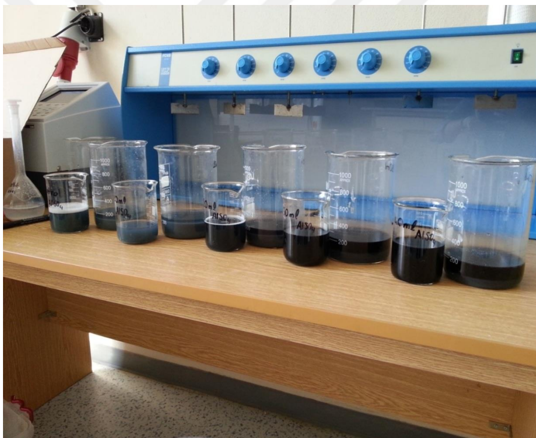
Figure 5.6 Jar testing kits and \text{Al}_2(\text{SO}_4)_3 application image
