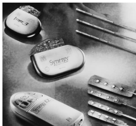
Figure 2.3 Neurostimulator and lead systems used for spinal cord stimulation to treat chronic pain. The Irel 3 and the Synergy are neurostimulators. The Synergy EZ is a patient programmer. Including percutaneous leads (top) and surgical leads (bottom) (Rise, 2000).
