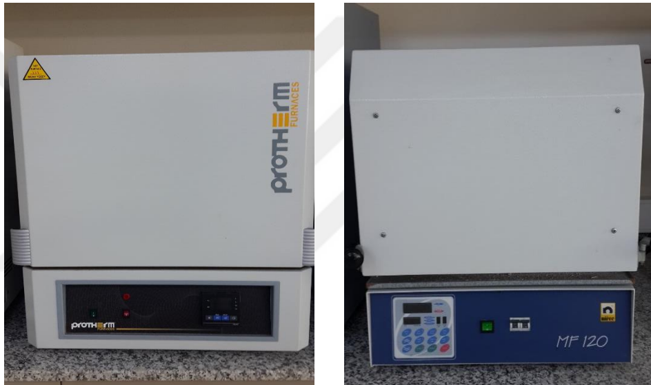
Figure 3.14 Protherm (metal oxide group) and Nüve MF120 oven (polymer) for heating processes
