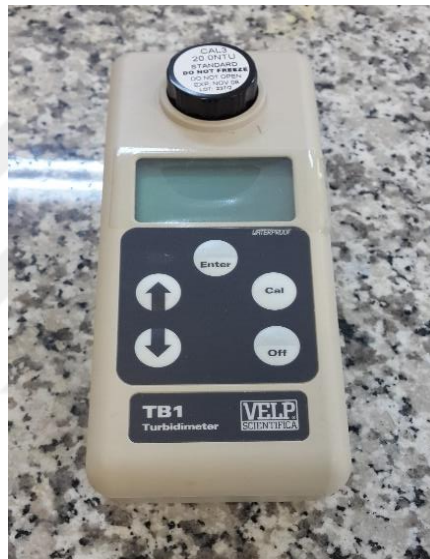
Figure 3.20 VELP TB1 turbidimetry
