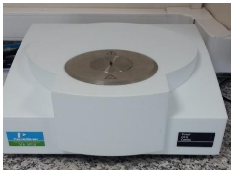
Figure 3.22 PerkinElmer STA 6000 Model Differential Thermal Analysis-Thermal Gravimetry
