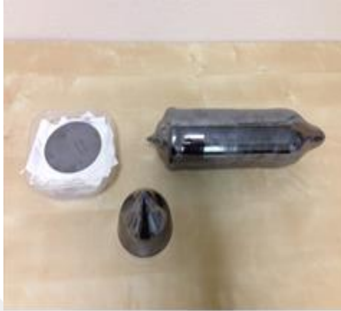
Figure 3.1 PVA Tepla Czochralski single crystal ingot and wafer
