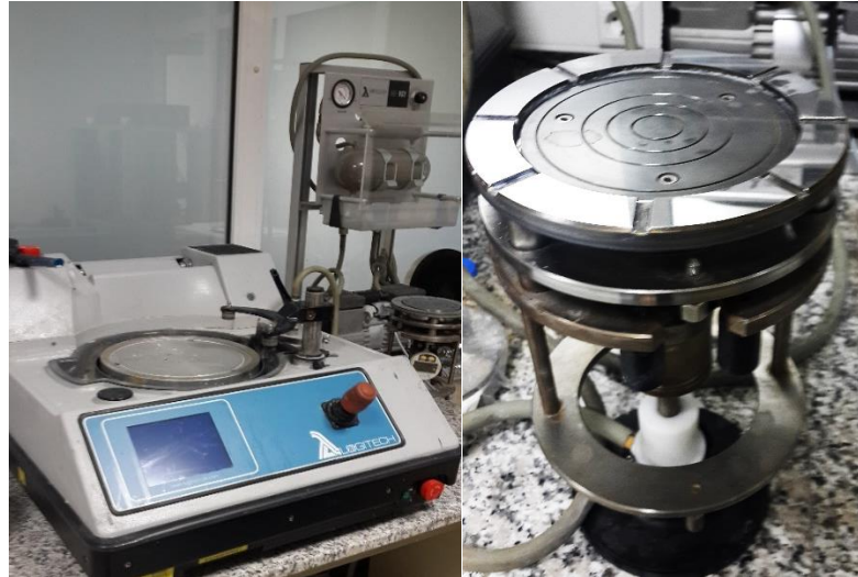
Figure 3.3 Slide silicon ingot lapping process
