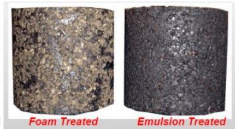
Figure 2.9 Foamed bitumen dispersion and binding in the treated mix
