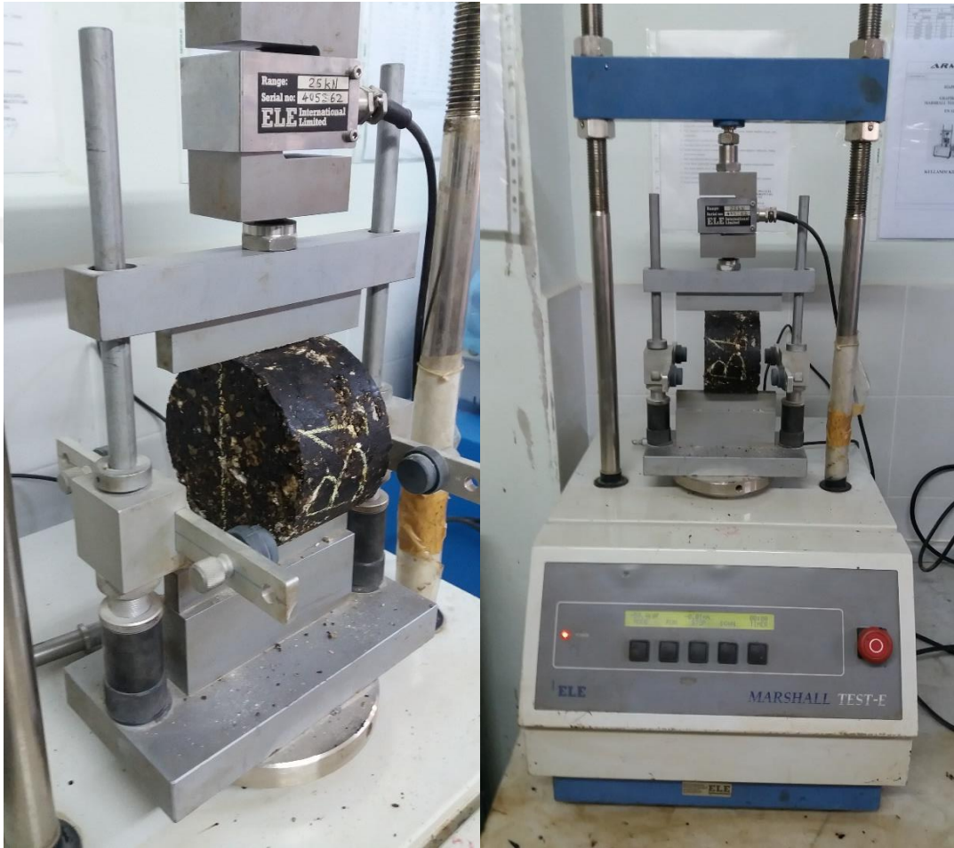
Figure 3.9 Indirect Tensile Strength (ITS) test of foam asphalt specimen
