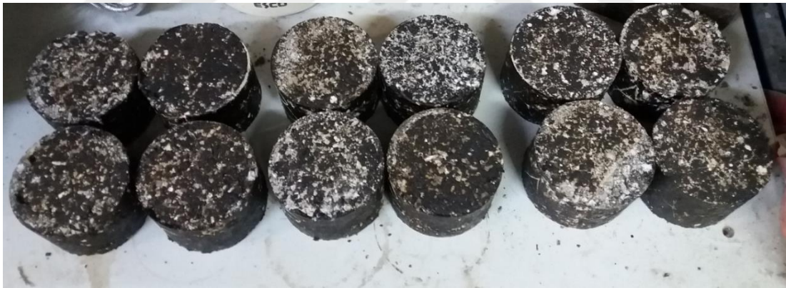
Figure 3.5 Foam asphalt specimens after compaction
