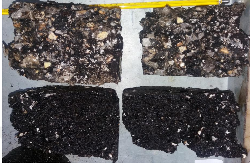
Figure 2.10 Aggregate particles coating in foam asphalt and hot mix asphalt Marshall Specimens
