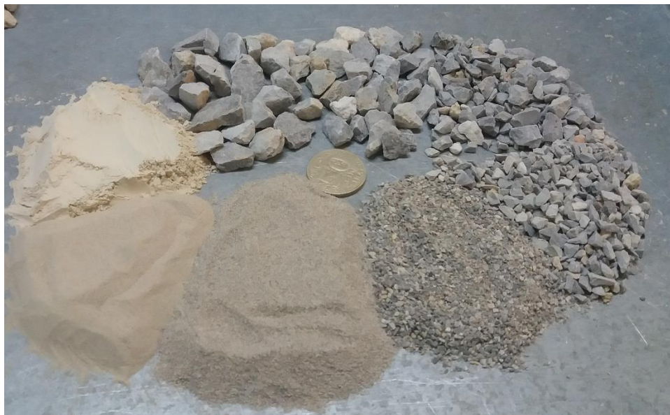
Figure 3.1 Aggregates particles sieved and separated according to size
