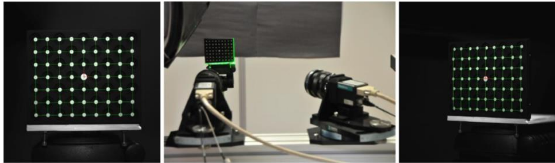
Figure 2.10 The calibration target with both cameras
