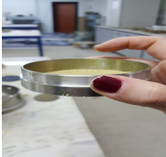
Figure 2.16 Pure bentonite sample prepared in height of 3 mm in the ring
