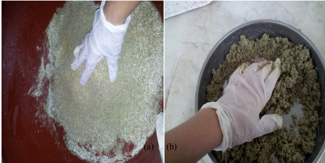
Figure 2.8 Kneading the mixture (a) Dry kneading, (b) Wet kneading
