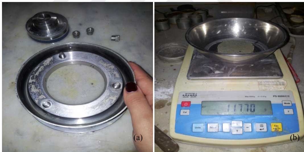
Figure 2.13 ZBM sample taken out of the cell and weighing for determination of water content a) ZBM sample after the test, b) Weighing the sample for water content
