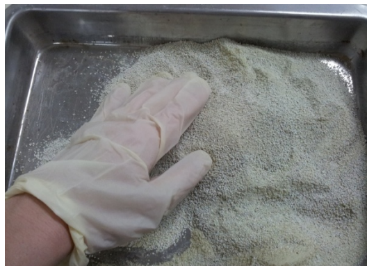
Figure 2.7 Dry mixing of zeolite and bentonite
