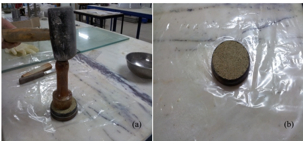
Figure 2.9 a) Placing the sample in the ring with help of mallet, b) Sample placed in the ring
