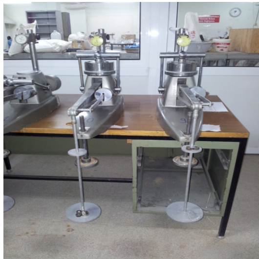
Figure 2.11 One dimensional consolidation test apparatus
