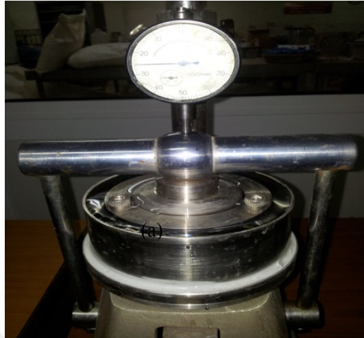
Figure 2.12 General view of the cell at the end of the swelling test
