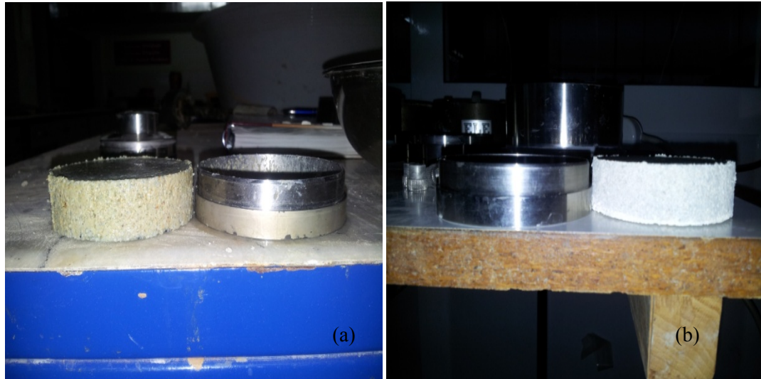
Figure 2.14 ZBM samples after completion of swelling (a) wet sample (b) dry sample
