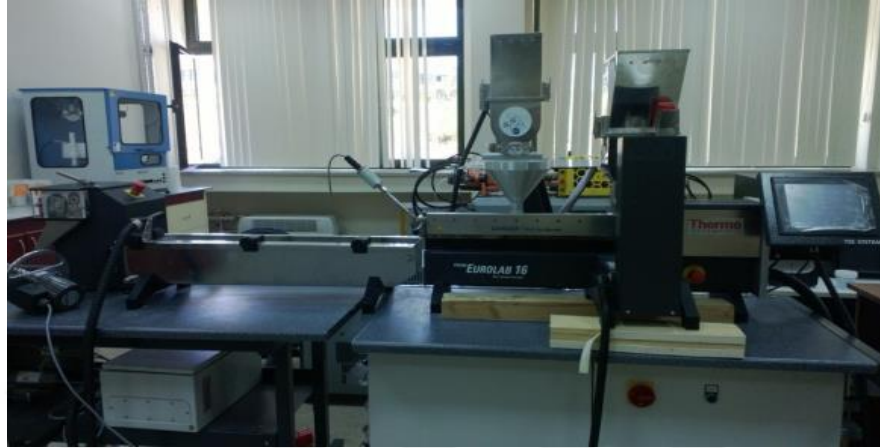
Figure 3.1 A co-rotating twin screw extruder
