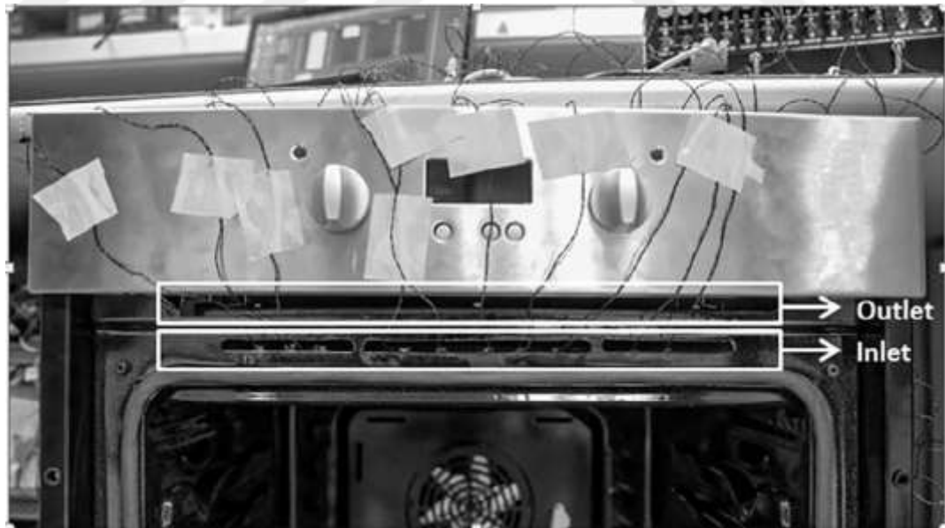
Figure 4.4 Arrangement of anemometers in experimental study (Personal archive, 2014)
