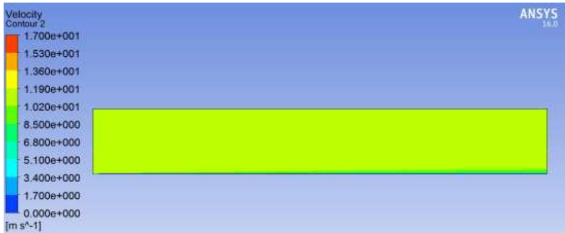
Figure 5.9 Velocity distribution map of the blade without droplet form add-on
