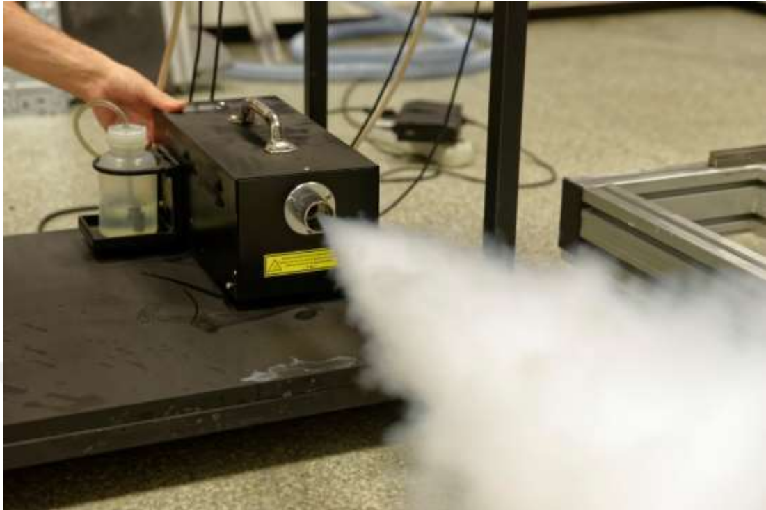
Figure 2.7 Photo of the current seed generator (Personal archive, 2017)
