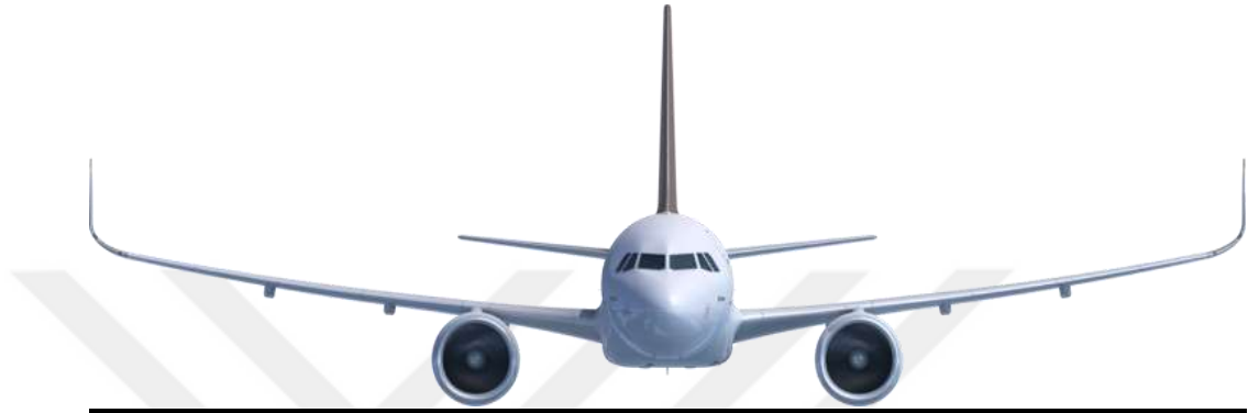
Figure 5.7 Form used on aircraft wings to break the tip vortex (www.airbus.com)
