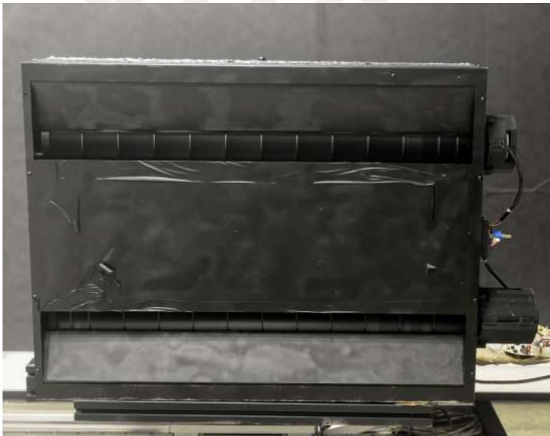
Figure 5.22 Front view of the prototype of the outdoor unit with CFF (Personal archive, 2016)
