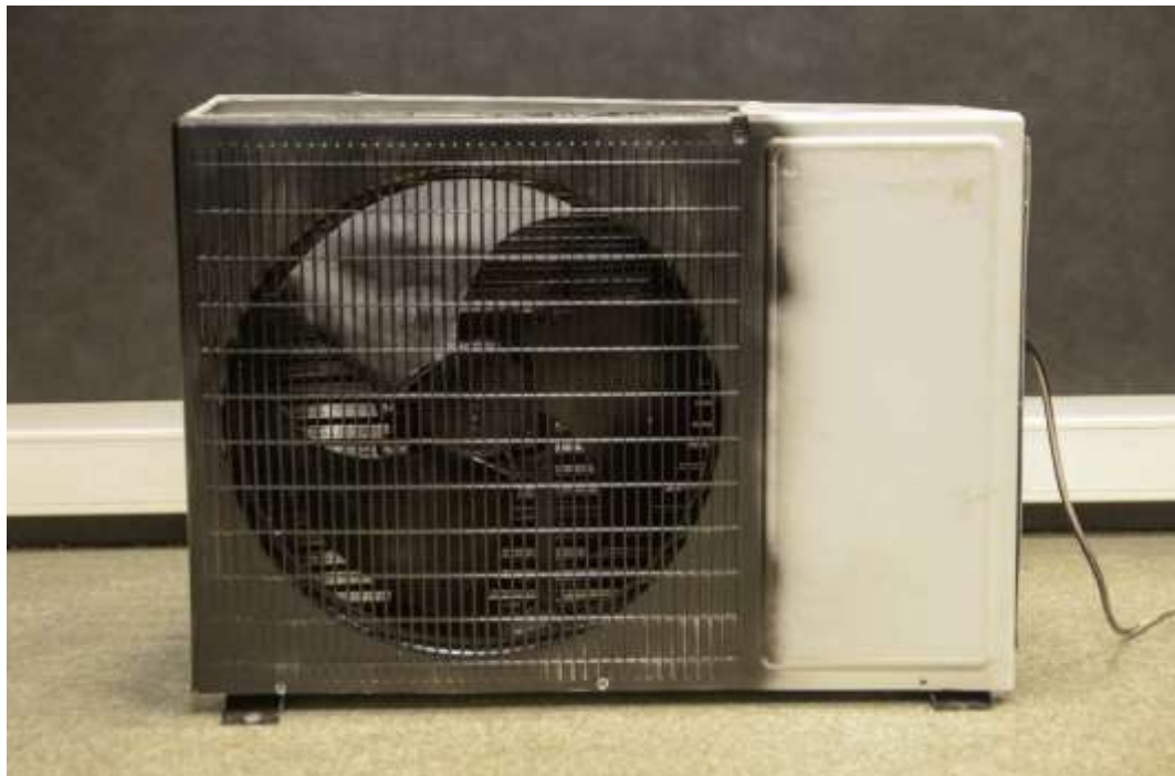
Figure 5.12 Final prototype of outdoor unit with axial fan (Personal archive, 2015)
