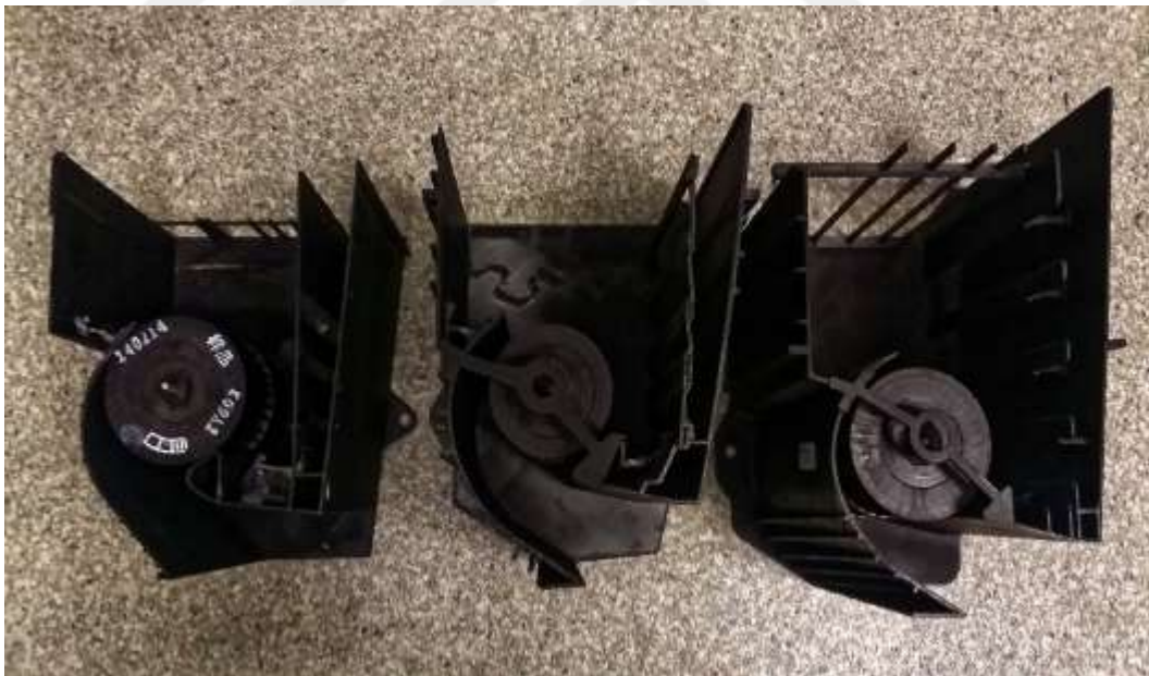
Figure 5.20 The CFF cut of prototypes used for endoscopic PIV (Personal archive, 2016)
