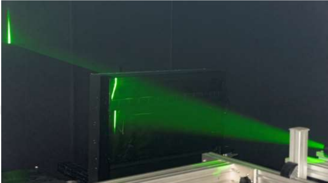
Figure 5.24 Investigation of prototype of outdoor unit with CFF by SPIV method (Personal archive, 2016)
