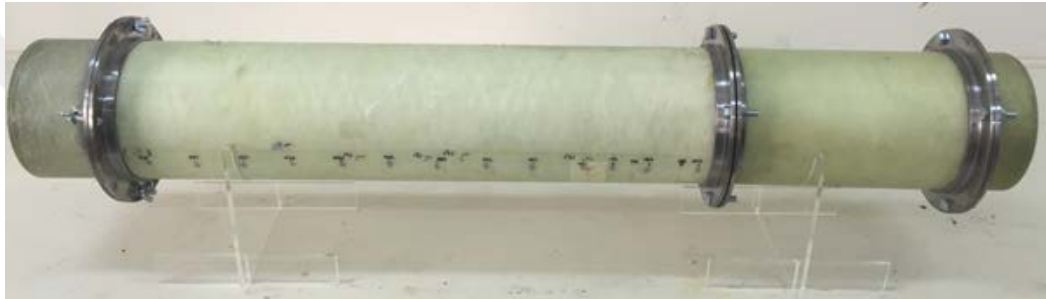
Figure 3.19 Low frequency sound absorption coefficient measurement tube kit of the “second prototype tube” (Personal archive, 2016)
