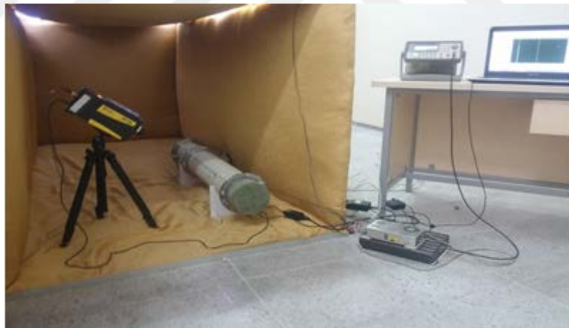
Figure 3.24 Outer surface impedance measurements setup (Personal archive, 2016)
