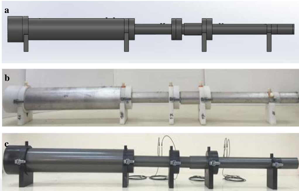
Figure 3.38 High frequency transmission loss measurement set (a: 3-D design model, b: manufactured system, c: painted system) (Personal archive, 2016)
