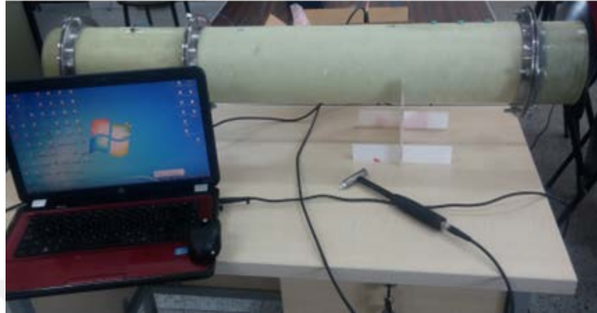
Figure 3.22 In situ modal test setup of the “second prototype tube” (Personal archive, 2016)
