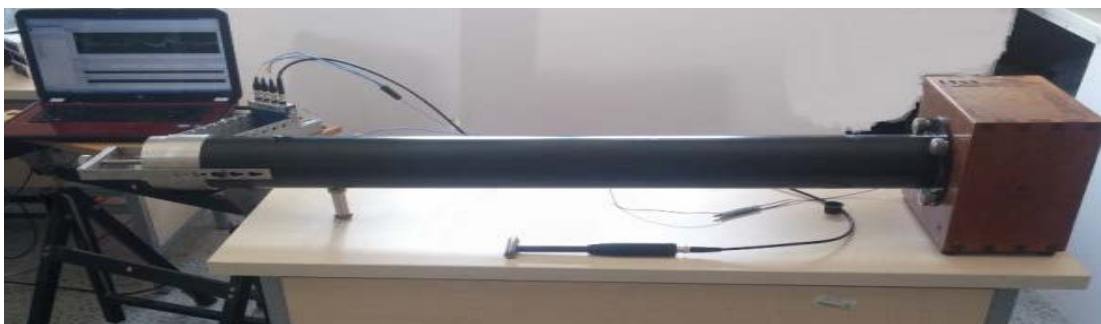
Figure 3.8 Experimental setup of in-situ structural modal analysis of brass tube (Personal archive, 2015)
