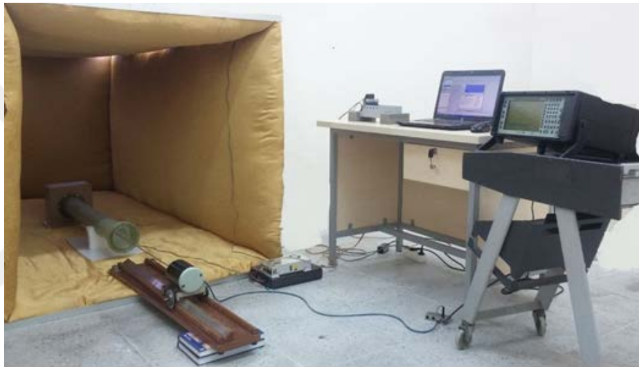
Figure 3.4 Experimental setup of acoustical modal analysis (Personal archive, 2015)
