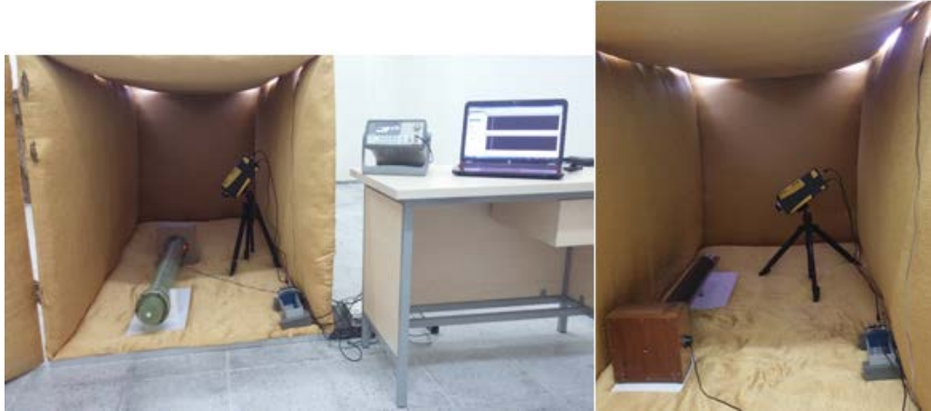
Figure 3.12 Experimental setup of outer surface impedance measurements (Personal archive, 2015)
