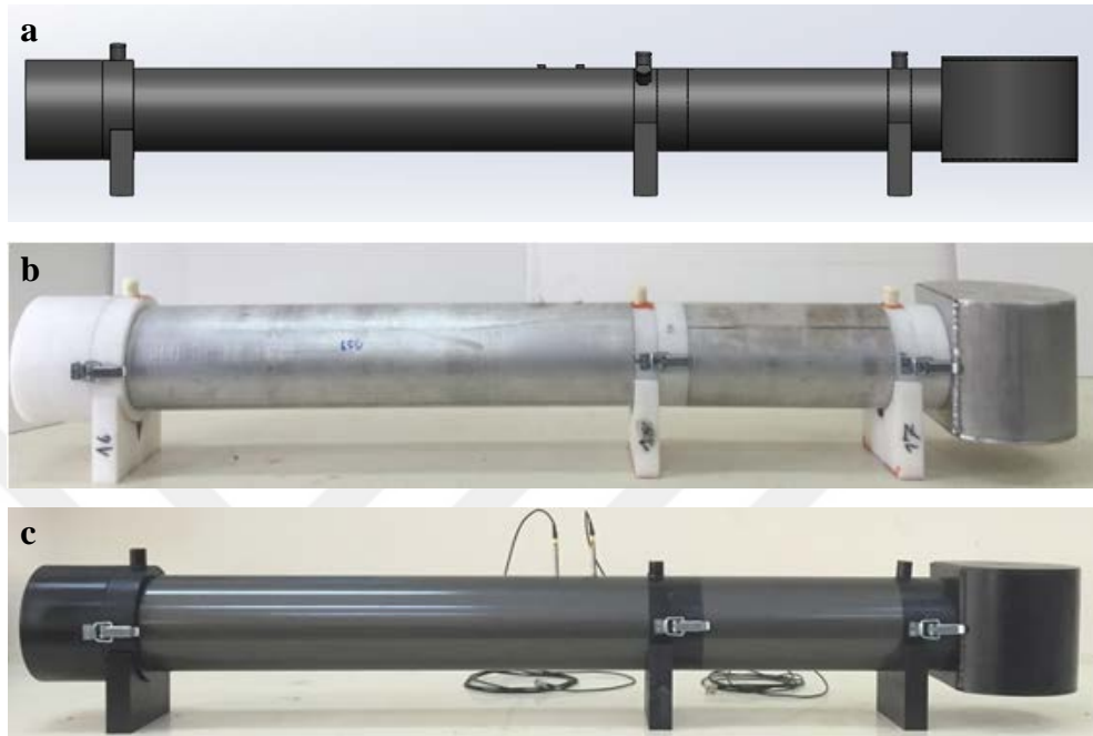
Figure 3.55 Rotation apparatus with low frequency sound absorption coefficient measurement set (a: design drawing b: manufactured system c: painted system) (Personal archive, 2016)
