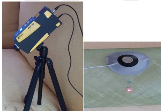
Figure 3.11 Laser vibrometer and surface microphone (Personal archive, 2015)
