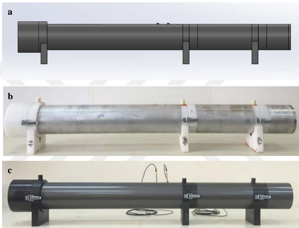
Figure 3.35 Low frequency sound absorption coefficient measurement set (a: 3-D design model, b: manufactured system, c: painted system) (Personal archive, 2016)
