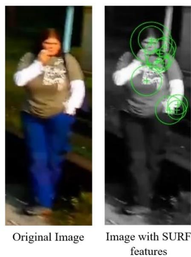
Figure 4.5 Visualization of SURF features
