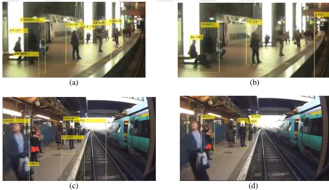
Figure 5.5 The detected bounding boxes(yellow), in the station departure scene with artificial lighting environment, by (a) HOG+SVM based model, (b) ACF+AdaBoost model and in another station scene with different angle of camera, by (c) HOG+SVM based model, (d) ACF+AdaBoost model
