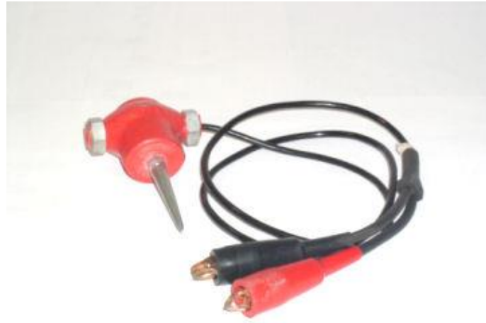
Figure 6.8 4.5 Hz vertical geophone (Geometrics, 2018)
