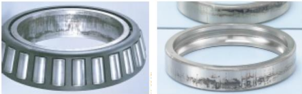
Figure 4.4 Wear and fretting failures (Koyo, 2015)
