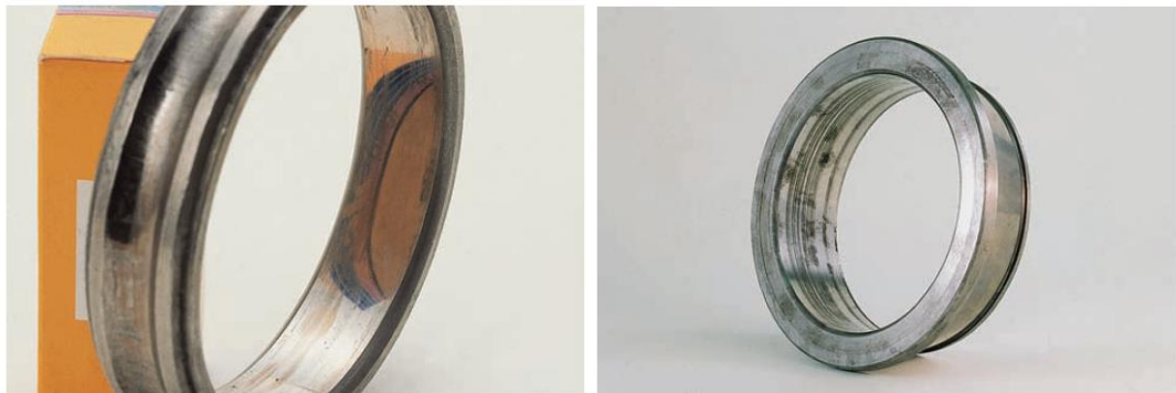
Figure 4.13 Creeping of inner rings (Barden, n.d.)
