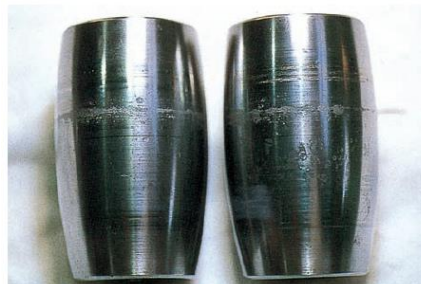
Figure 4.3 Peeling on rolling contact surfaces (Action Bearing, n.d)
