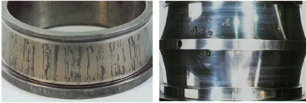
Figure 4.8 Corrosion of bearing rings (NTN, 2017)
