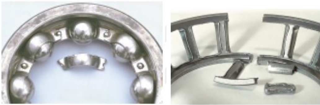
Figure 4.11 Examples of cage damages (Koyo, 2015)
