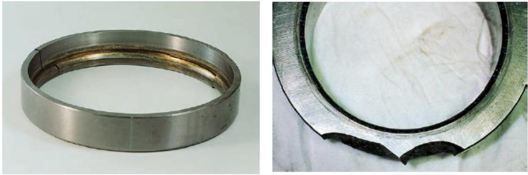
Figure 4.5 Cracks and chips failures (Action Bearing, n.d)
