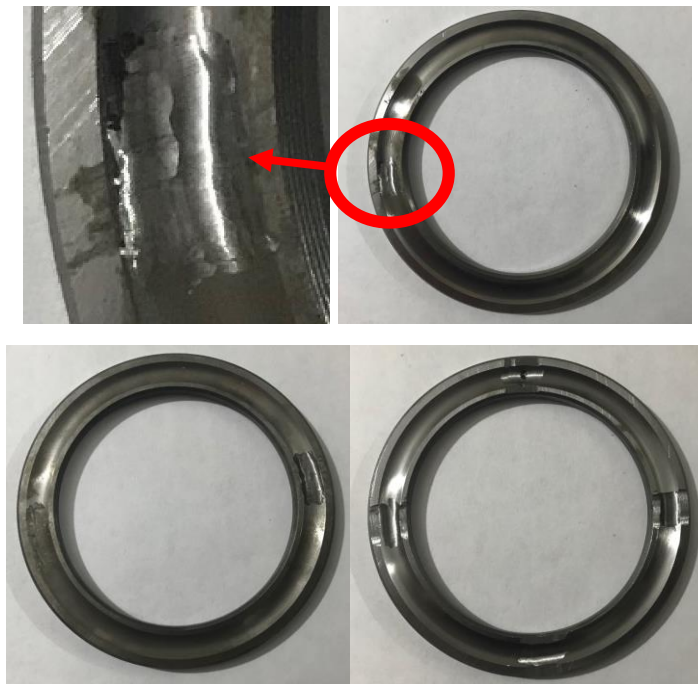
Figure 5.8 Housing washers of thrust bearings that defect generated (Personal archive, 2019)
