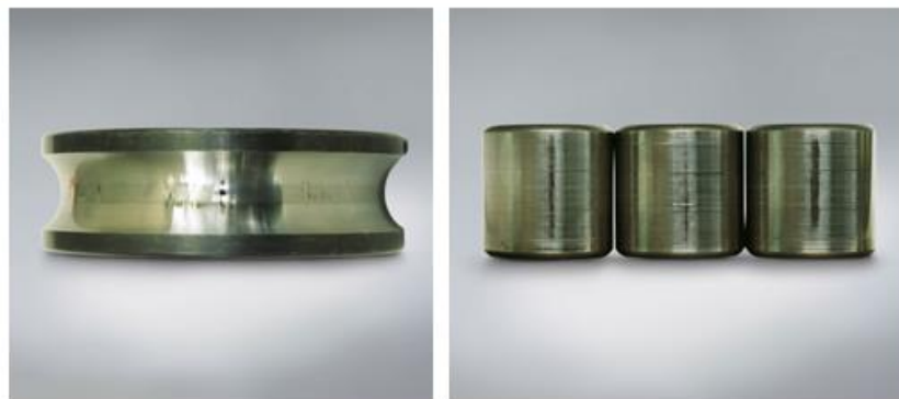
Figure 4.5 Examples of brinelling (Action Bearing, n.d)
