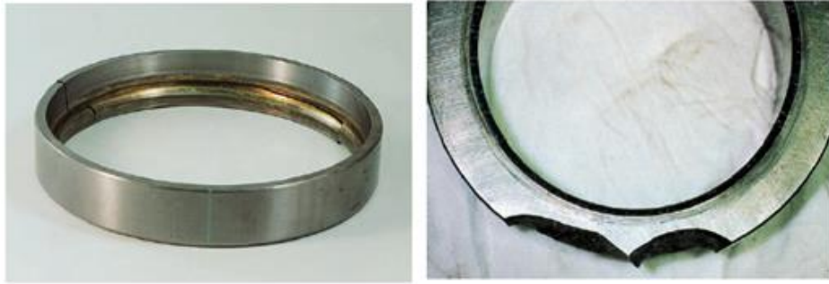
Figure 4.3 Cracks and chips defects (Action Bearing, n.d)
