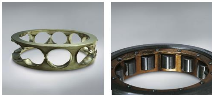
Figure 4.4 Examples of cage damages (Koyo, 2015)
