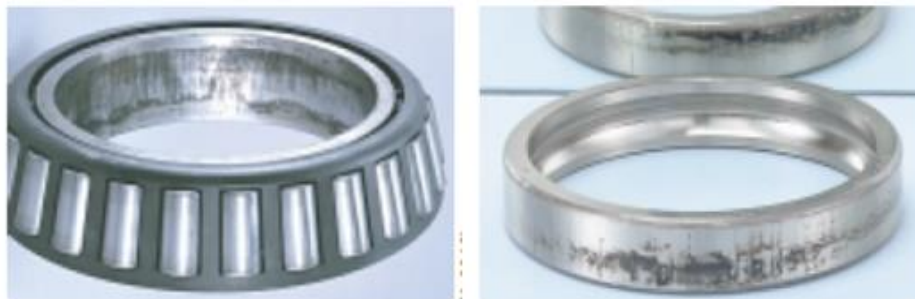
Figure 4.7 Wear and fretting failures (Koyo, 2015)
