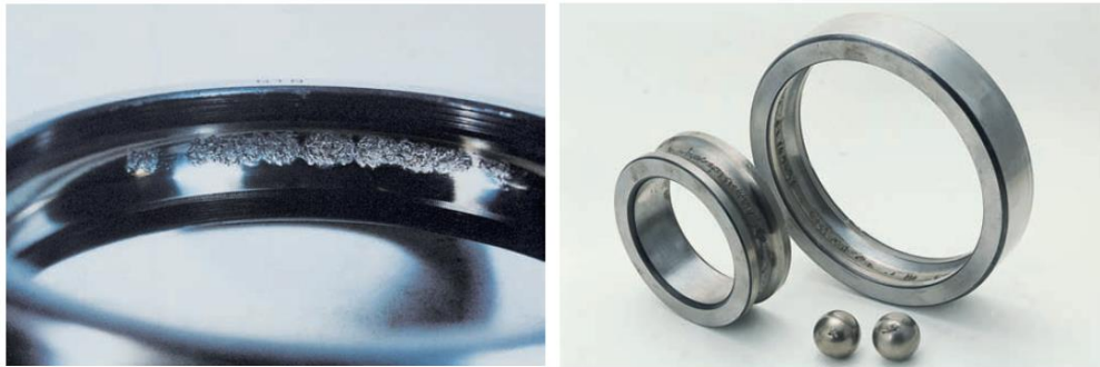
Figure 4.2 Inner ring, outer ring and balls are flaked (NTN, 2017)
