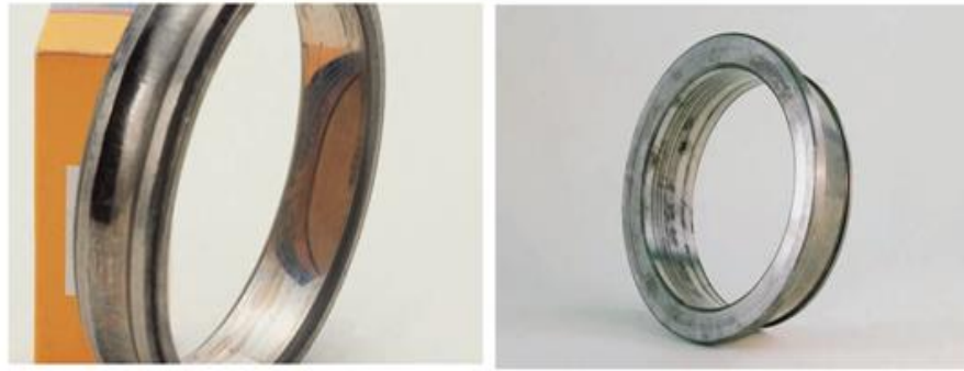
Figure 4.6 Creeping of inner rings (Barden, n.d.)
