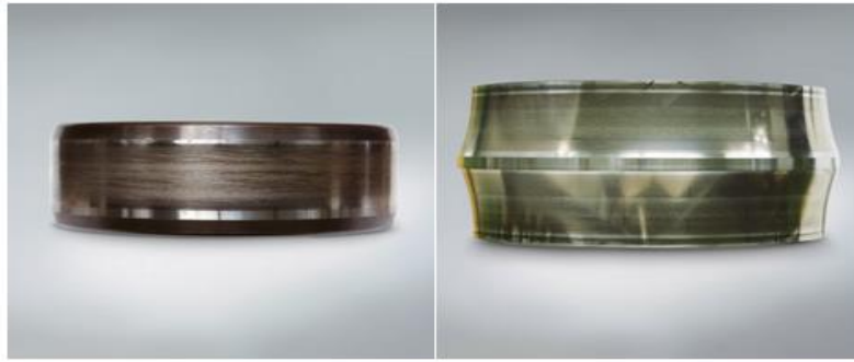
Figure 4.9 Examples of smearing damage (NTN, 2017)
