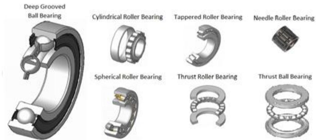
Figure 2.10 Types of rolling elements (SDP/SI, 2018)
