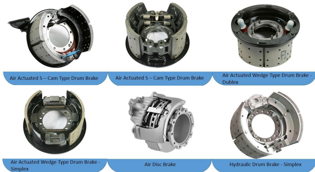
Figure 5.1 Complete brake groups (Egefren, n.d.)
