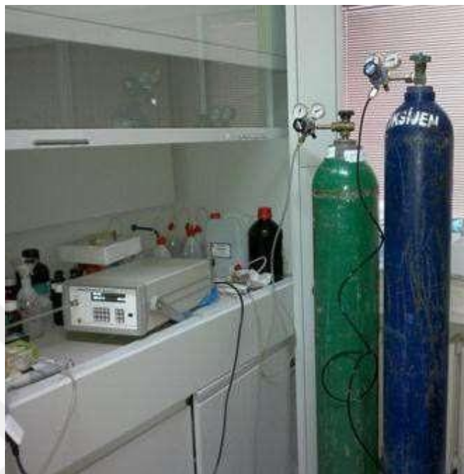
Figure 2.12 Gas blender instrument and oxygen and nitrogen cylinders (Personal archive, 2019)
