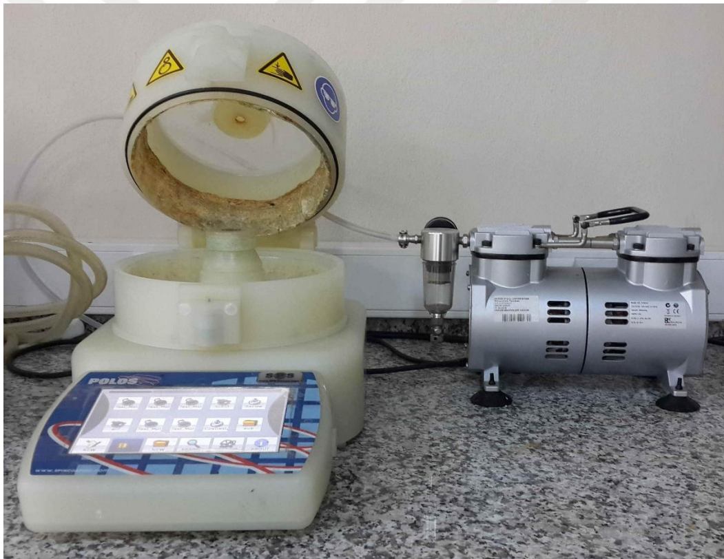
Figure 2.14 Spin coating device (Personal archive, 2019)
