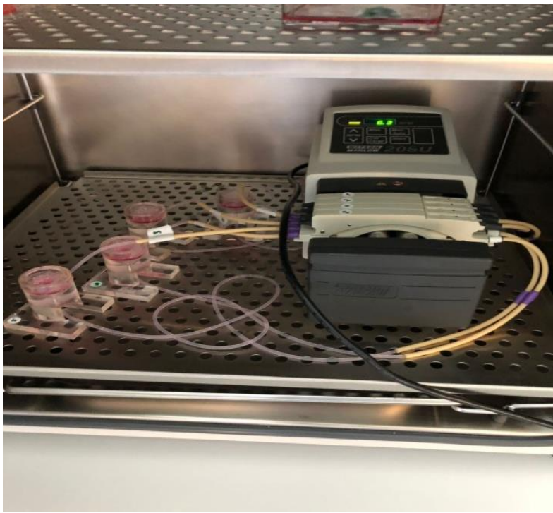
Figure 2.2 Fluidic Shear Stress Treatment. Watson Marlow 205U peristaltic pump, Marprene Tube Elements for 2.79 bore Watson Marlow tubing and bubble traps were used.
