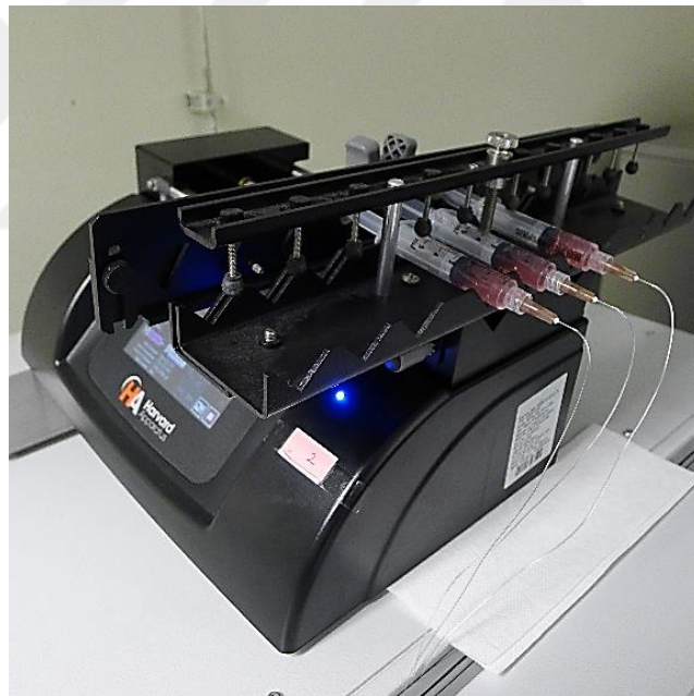
Figure 18: Connected syringe pump on top of a culture incubator.
