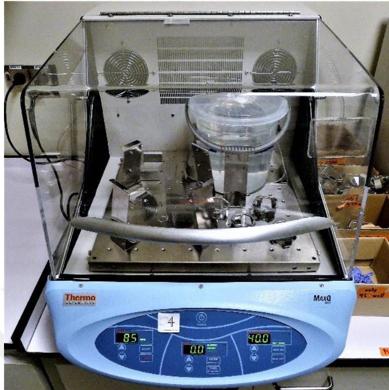
Figure 3: GelMA dialysis step taking place in orbital shaker.
