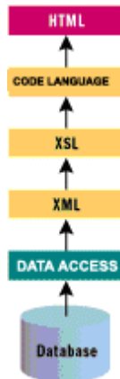
Figure 4.19 Concept diagram for XML/XSL data presentation approach
