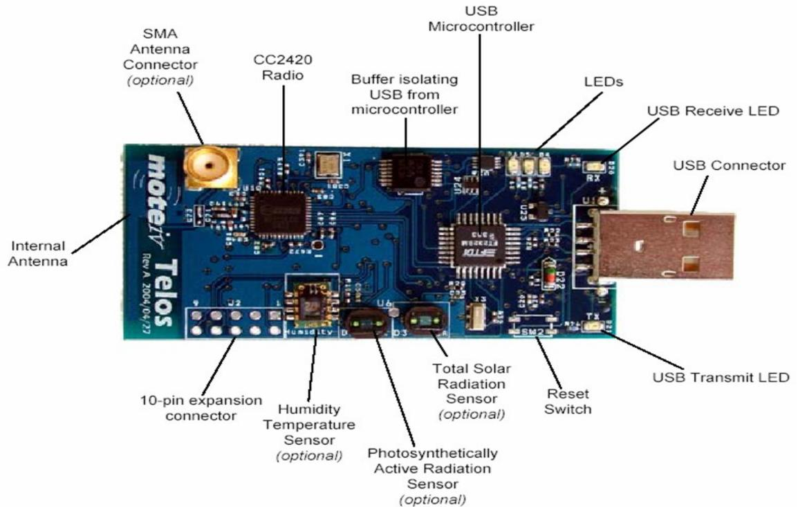
**Figure 2.2 : TMote-Sky node used in channel modeling at smart grid environments**
