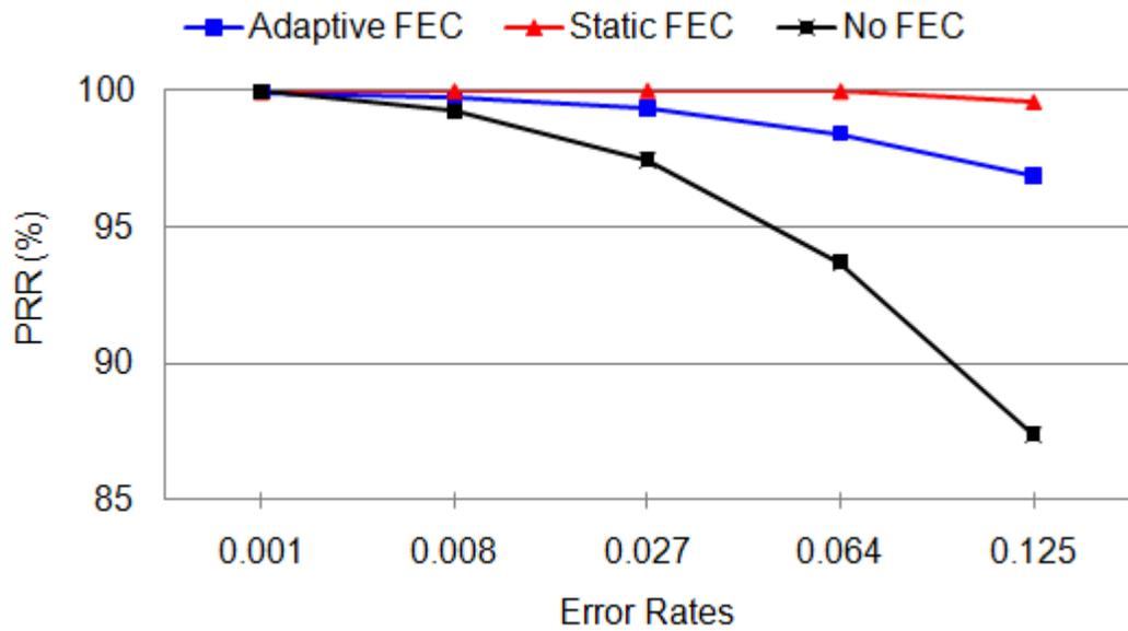
Figure 4.6 : PRR vs. error rates in outdoor 500 kV substation
