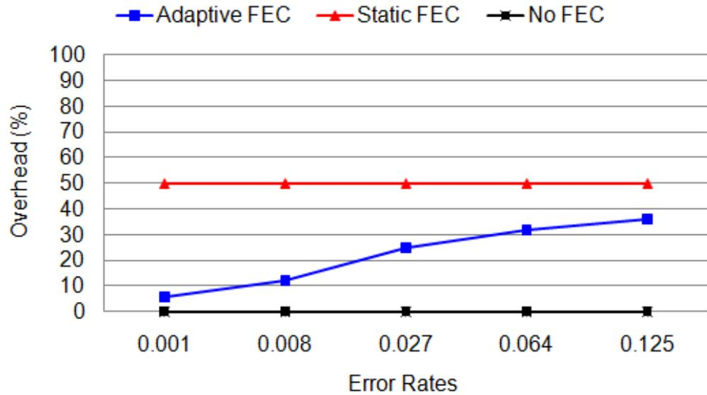
Figure 4.4 : Overhead vs. error rates in outdoor 500 kV substation
