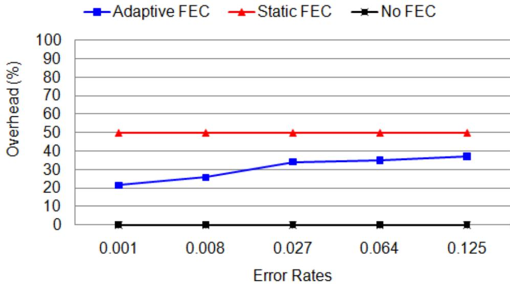
Figure 4.5 : Overhead vs. error rates in underground transformer vault
