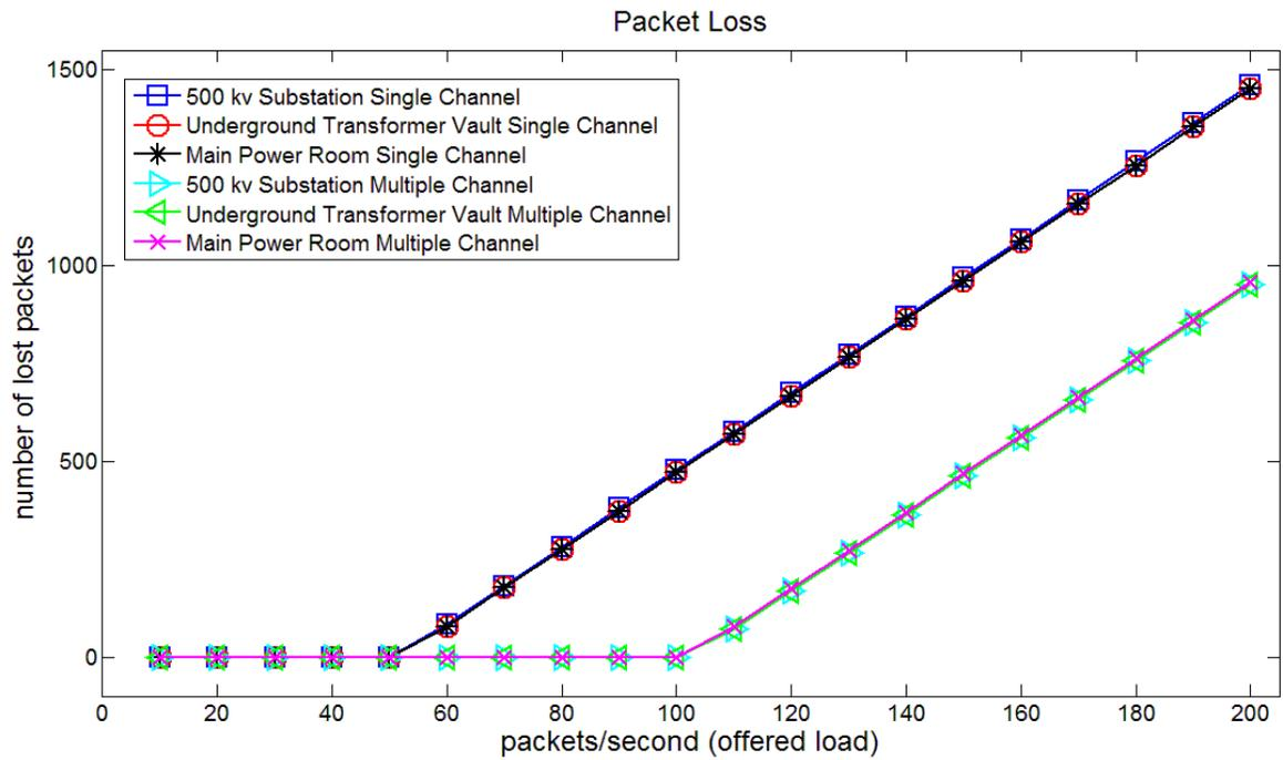
**Figure 5.4 : Packet loss vs. number of transmitted packet**
