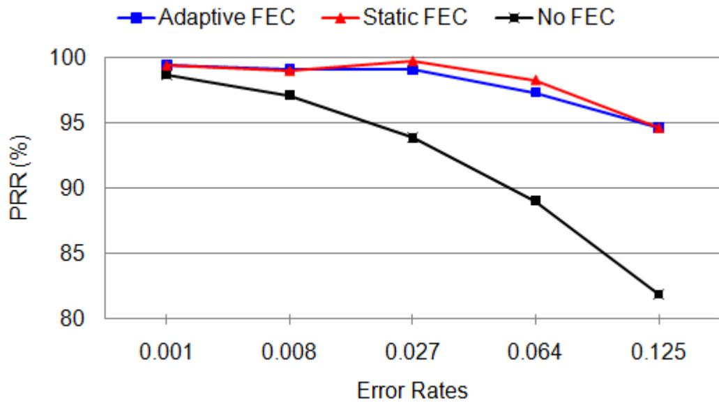
Figure 4.7 : PRR vs. error rates in underground transformer vault
