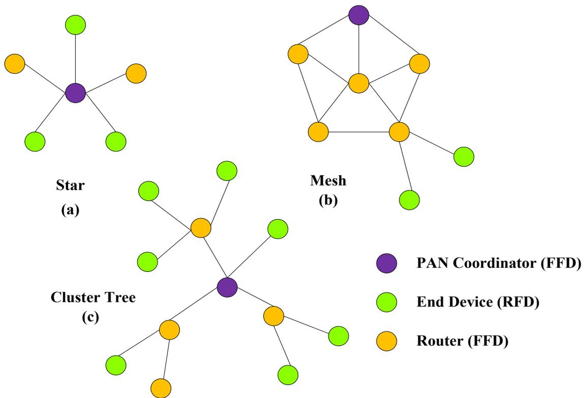
**Figure 3.2 : Network topologies a) star topology, b) mesh topology, c) cluster tree**
