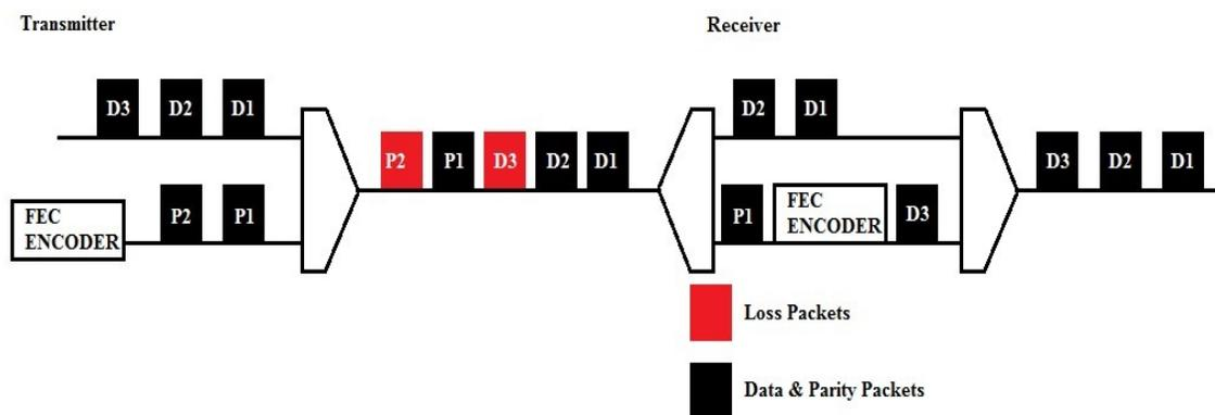
**Figure 4.2 : Static FEC mechanism**
