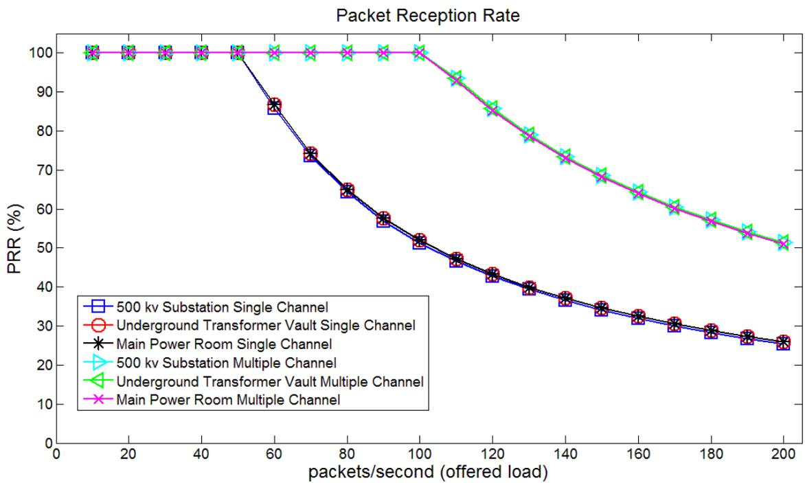
**Figure 5.3 : Packet reception rate vs. number of transmitted packet**
