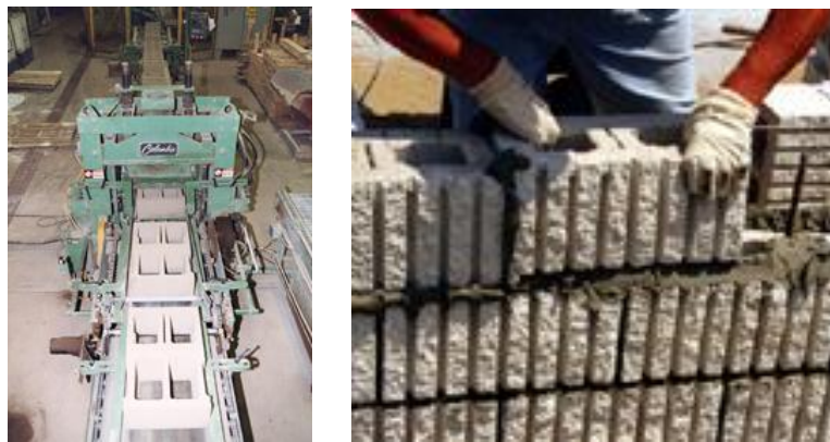
Figure 4.18: A modern block plant in operation and its application in site
