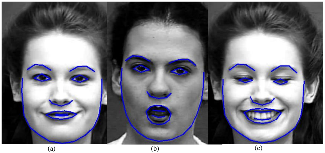
Figure 3.14: Some mistakes of Stasm method (a) Stretched lips. (b) Mouth is bigger than expected. (c) Although the eyes are closed they are drawn as if they are open
