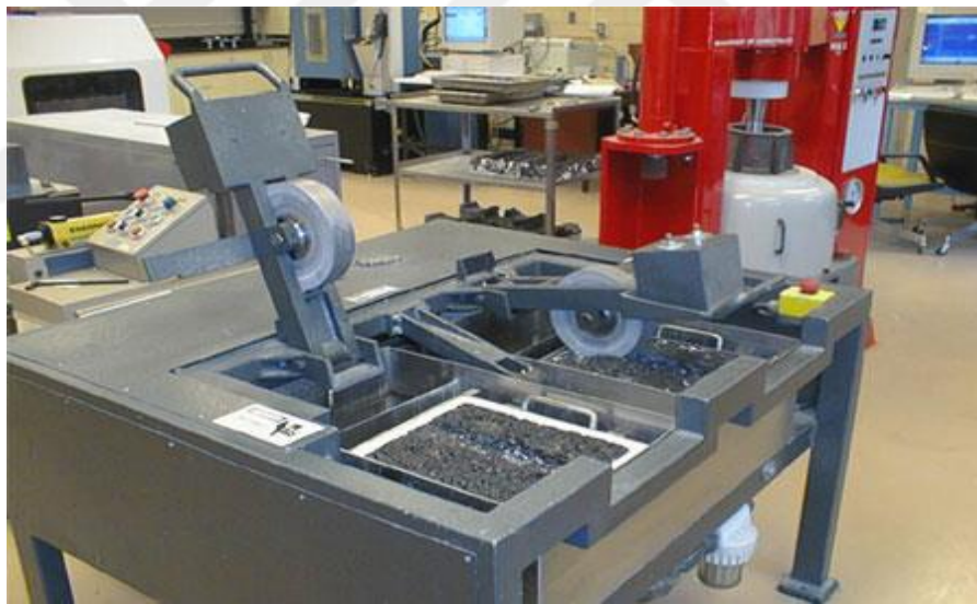
Figure 5.13. Hamburg wheel tracking device [70].
