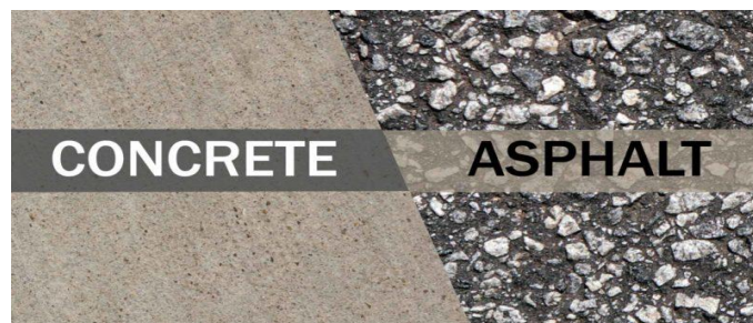
Figure 3.1. Flexible pavement and rigid pavement [47].
