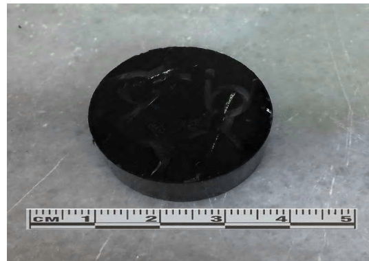
Figure 3.9. Hot mounting ribbon sample
