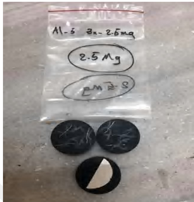
Figure 3.12. The MS ribbons and CS samples after hot mounting and polishing
