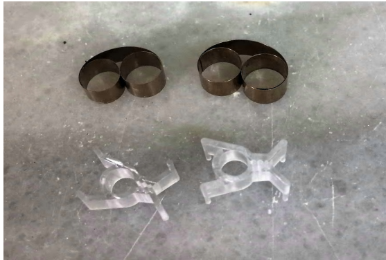
Figure 3.8. Hot mounting process clips
