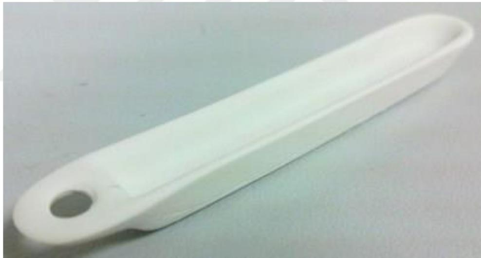
Figure 3.3 Alumina crucible
