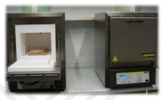
Figure 3.2. Furnaces used for solid state reactions
