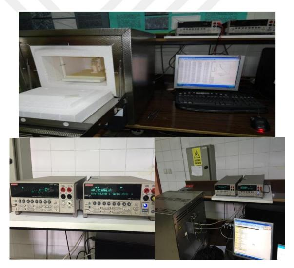
Figure 3.9. Computer controlled electrical conductivity measurement system
