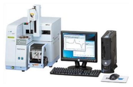
Figure 3.7. Image of the Perkin Elmer DTA/TG measurement system
