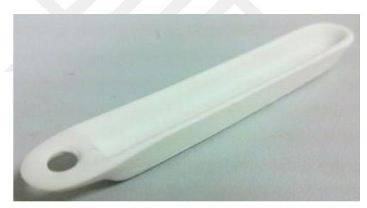
Figure 3.3 Alumina crucible
