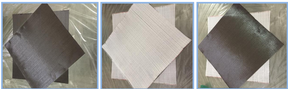
Figure 3.1. Specimens preparing: (a) carbon fibers, (b) E-glass fibers, (c) hybrid.
