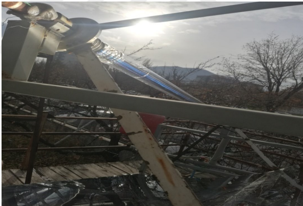
Figure 2. 14 The reflected radiation focused on tube receiver.
