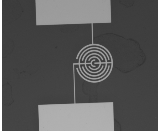
Figure 3.15. The patterned (etched) glass substrate view under optical microscope
