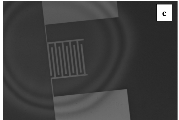
Figure 3.7. ITO deposited thin film device (a) cross sectional (b) schematic view under the optical microscope (c) Physical ITO deposited device under microscope
