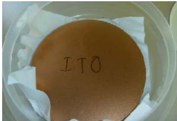
Figure 3.5. 14 cm 99.99% purity ITO target
