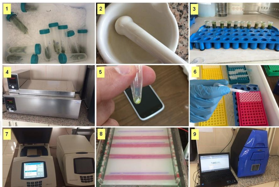
Figure 3.7. Image (1-6)Steps of genomic DNA isolation, Image (7) production of amplified DNA templates, using (PCR) instrument. Image (8) transferring the amplified DNA by 2% agarose gel electrophoresis methods. Image (9) recording and modifying obtained Images by UV (MS.Major Science) visualizing system
