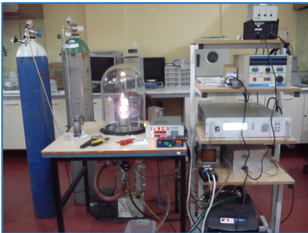
Figure 3.2. The home-build RF-MS system used
