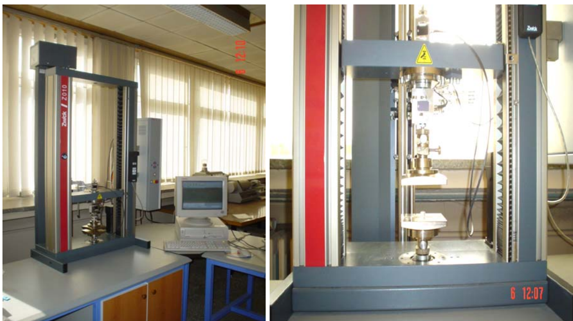
Fig. 5.1. The photographs of Universal Testing Machine and uniaxial compression module.
