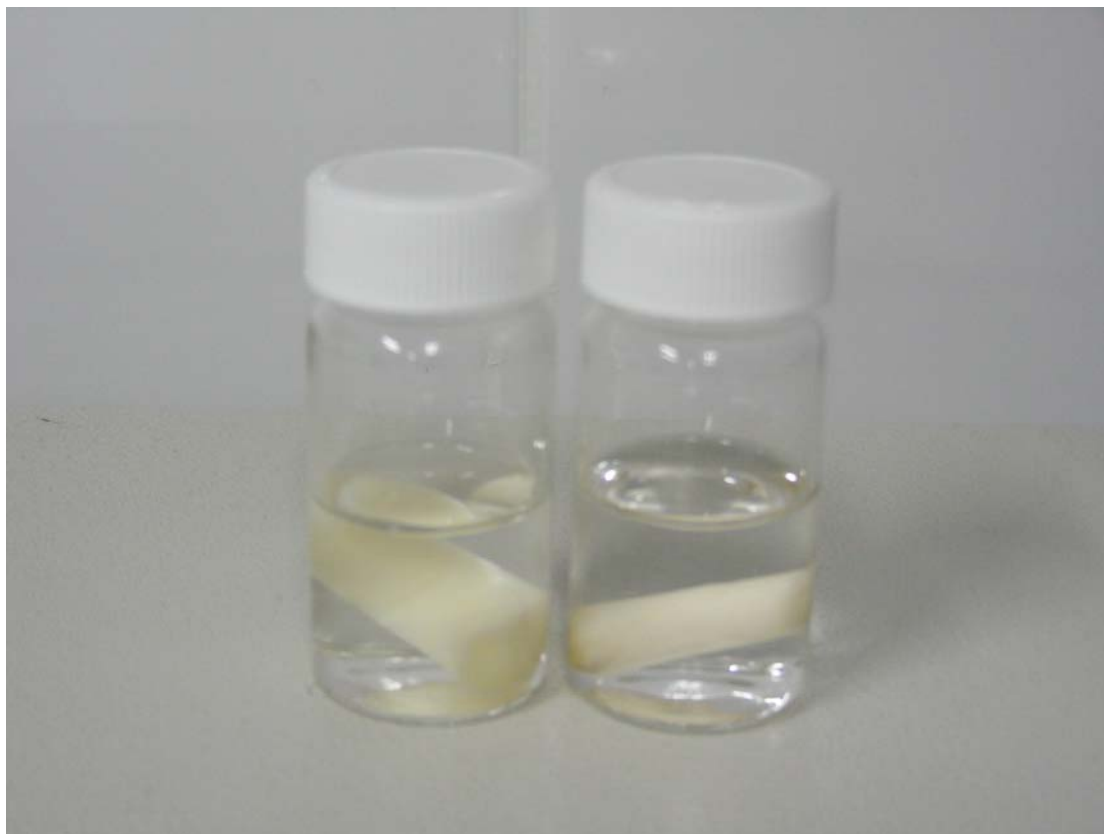
Figure 4.3. Digital photograph of the template removed poly(NIPA-MAC) gels below (22°C) and above (38°C) at LCST temperature.
