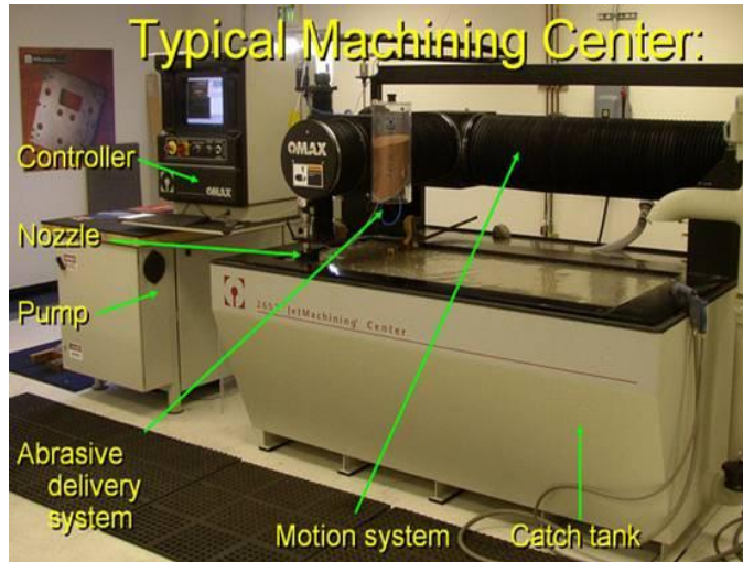
Figure 2.7. Typical Machining Center (Agus et al..1996)
