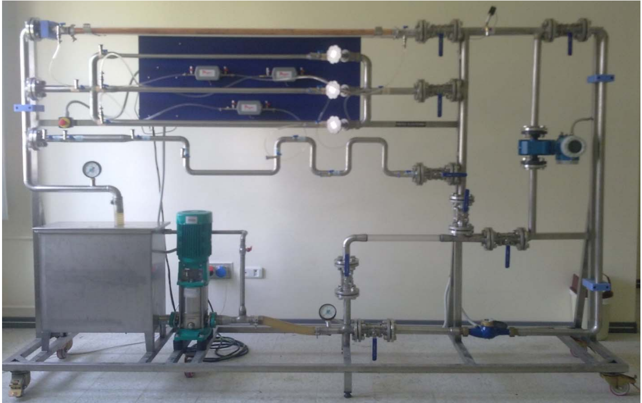
Figure 4.1. The experimental setup for basic fluid mechanics applications
