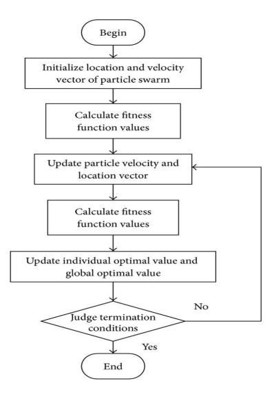
Figure 2.18. Flowchart of PSO algorithm
