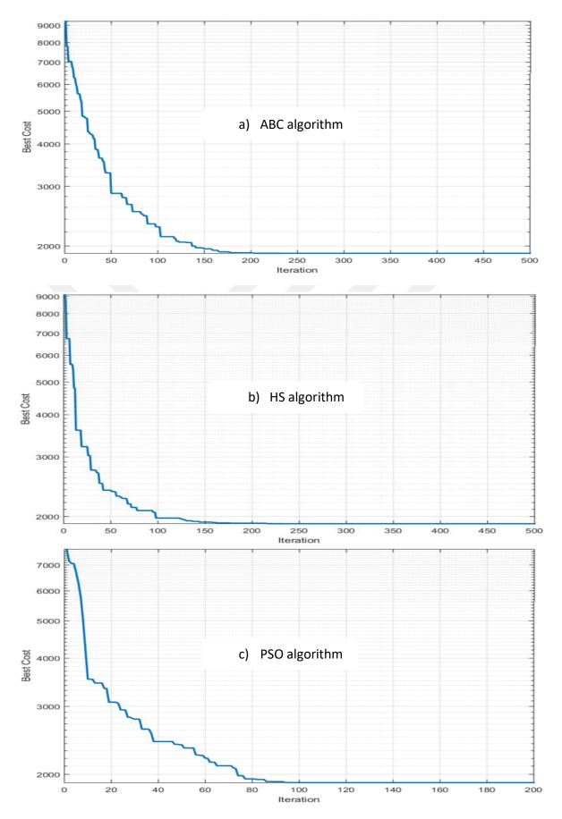
Figure 3.10. Convergence histories for 52-bar planar truss structure
