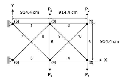
Figure 3.2. 10-bar planar truss structure
