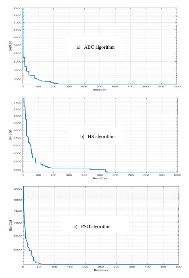
Figure 3.3. Convergence histories for 10-bar planar truss structure (case 1)
