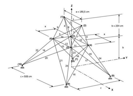
Figure 4.2. 25-bar spatial truss structure
