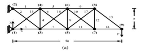
Figure 3.5. 17-bar planar truss structure, a = 254cm (100 in)
