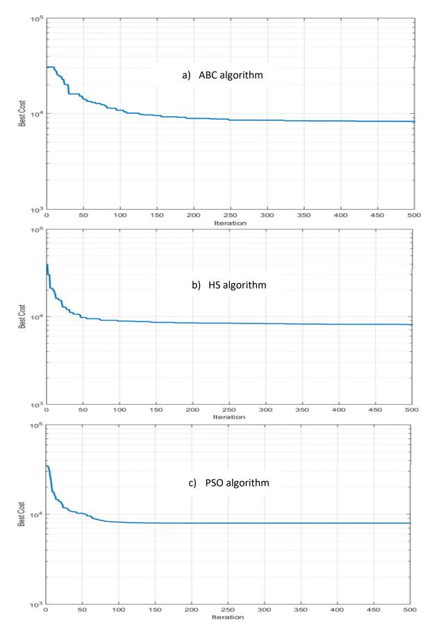
Figure 3.8. Convergence histories for 45-bar planar truss structure
