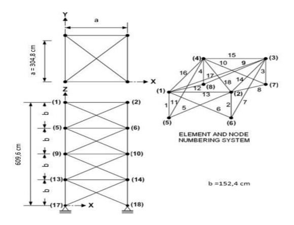
Figure 4.4. 72-bar spatial truss structure
