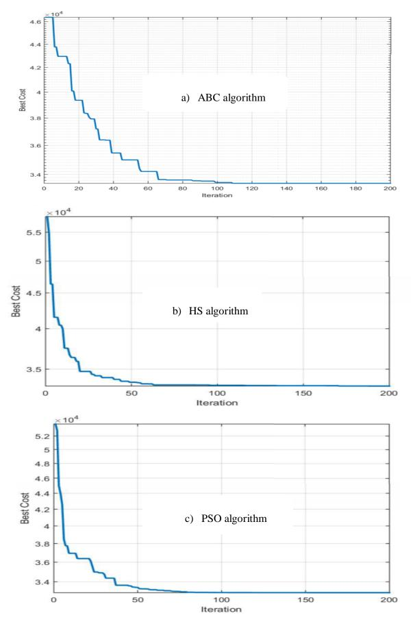
Figure 4.8. Convergence histories for 120-bar spatial truss structure (case 2)
