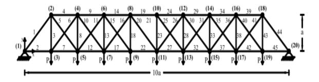
Figure 3.7. 45-bar planar truss structure, a = 508 cm (200 in)
