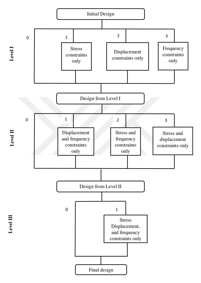
Figure 2.3. Optimality criteria code levels and constraint inclusion strategies
