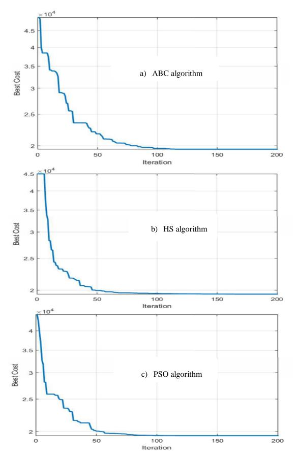
Figure 4.7. Convergence histories for 120-bar spatial truss structure (case 1)
