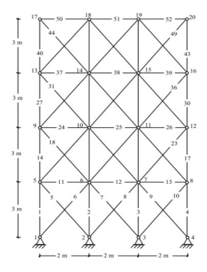
Figure 3. 9. 52-bar planar truss structure
