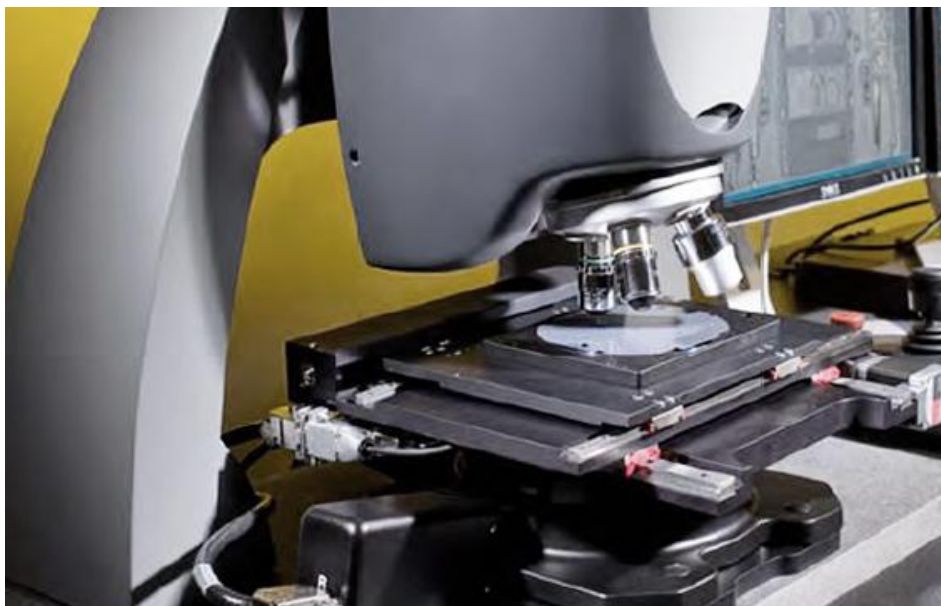
Figure 4.8 Zygo- Newview 7200 optic profilometer (NNRC).
