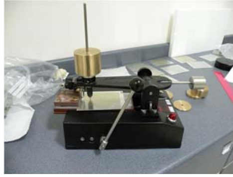
Şekil 3.11 Sheen Instruments-706 Hand Scratch Tester
