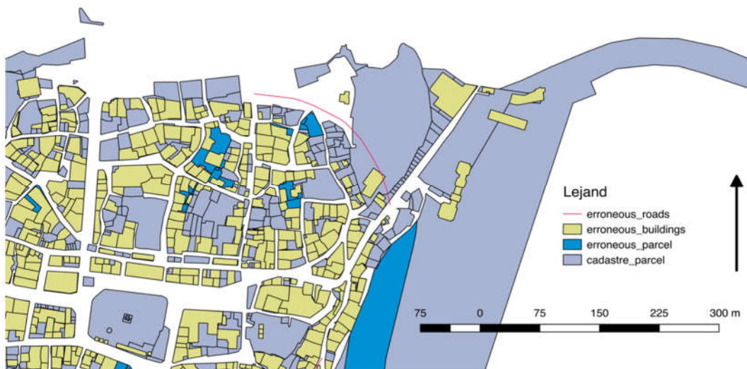
Figure 64. Erroneous features. Red road crosses with the yellow buildings.
