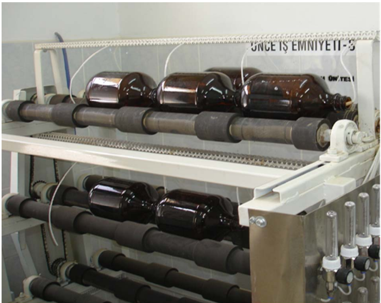
Figure 2.6. Bottle Roll Test Machine
