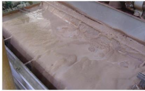
3.6x3.6 meter (12x12 ft) CrossFlow Separator for the classification of potash prior to a split feed flotation circuit.
