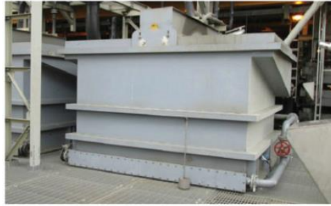
2.2x2.2 meter (7x7 ft) CrossFlow Separator for the recovery of fine tungsten.
