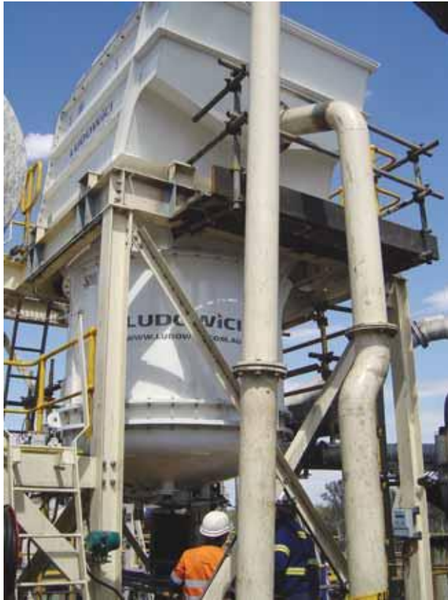
Figure 12. Diagram representing a Reflux Classifier.
