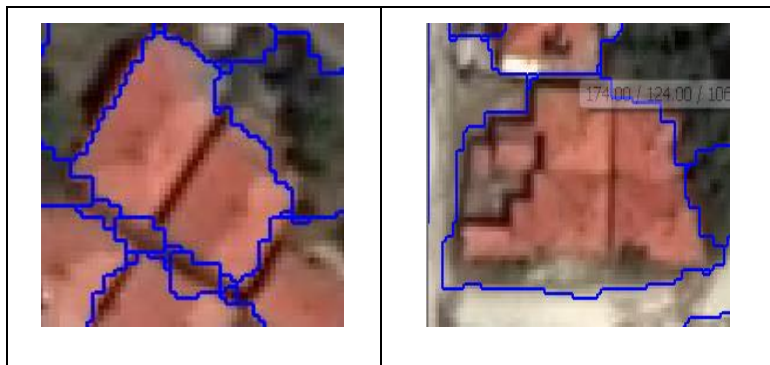
Figure 4.4. The merged segment of the adjacent roofs
