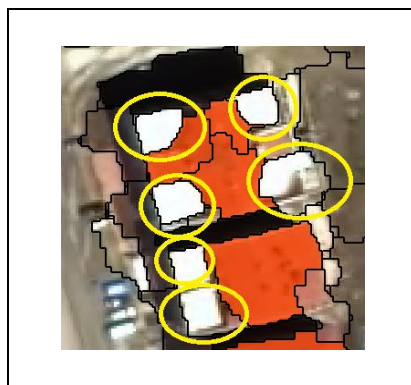
Figure 4.15. Building roofs with white areas. These white areas on the roof were segmented as different image objects and they were not classified as building
