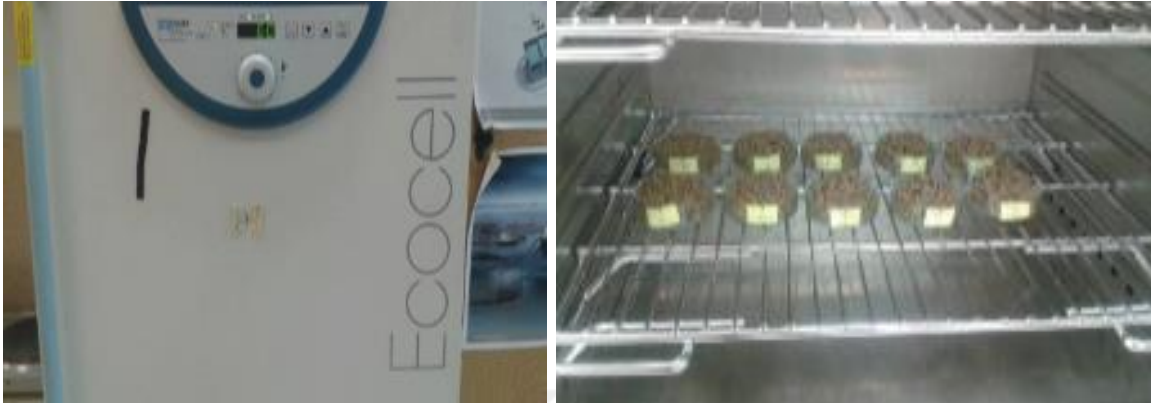
Figure 3. Uneaten pellets collected from individual tanks were dried in an Ecocell Drying Oven
