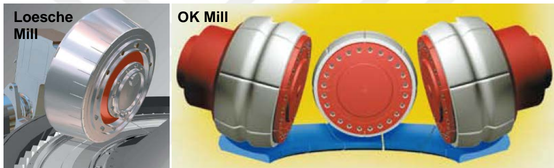
Figure 2.31 The roller and grinding table profile [39,42]
