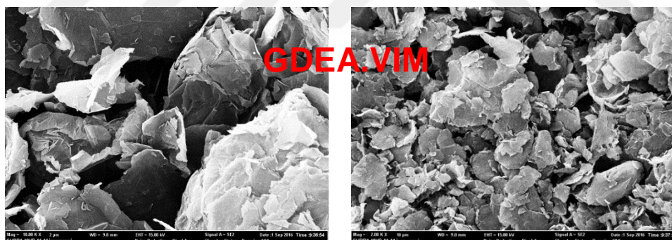
Figure 4.63. SEM images of DEA-modified graphene – VIM composites
