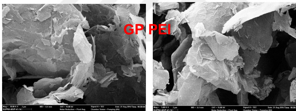
Figure 4.60. SEM images of H 3 PO 4 -modified graphene – PEI composites
