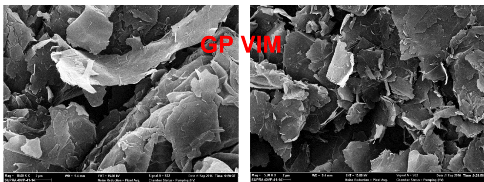
Figure 4.61. SEM images of H 3 PO 4 -modified graphene – VIM composites
