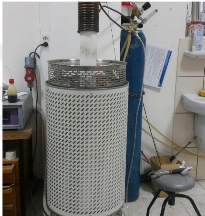
Figure 15 Conventional sintering furnace and high purity argon-filled tube
