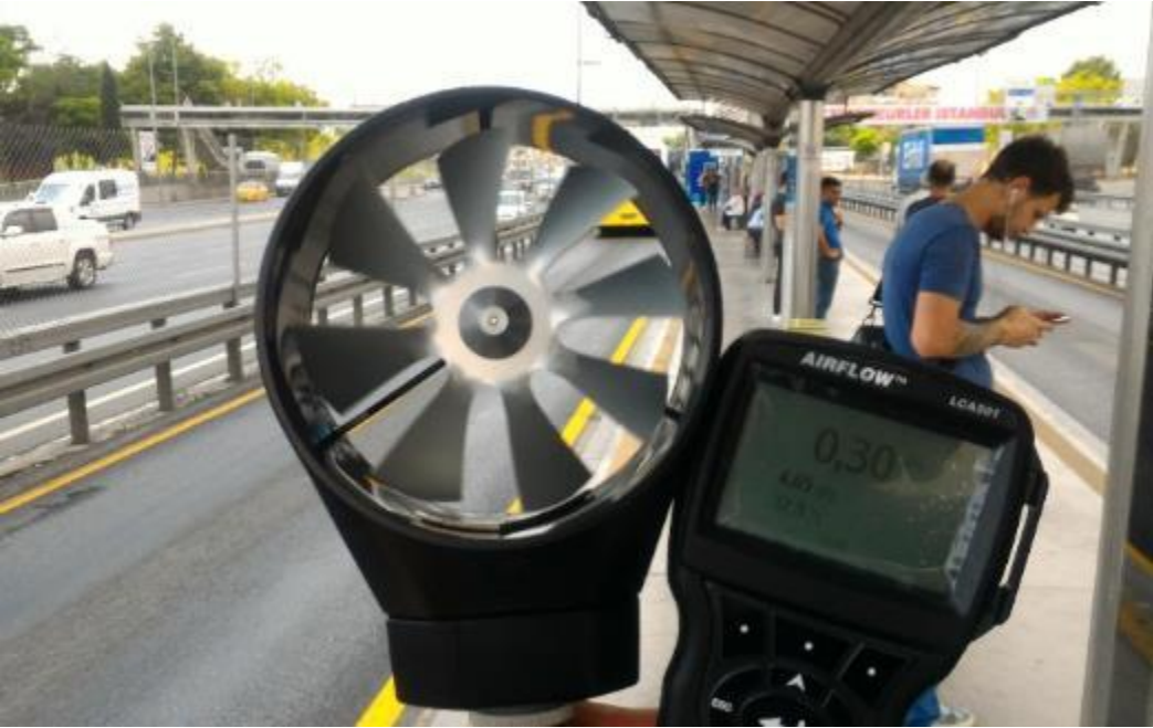
Figure 3-7 Wind speed measurement
